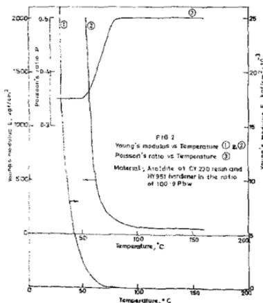
FIG. 1. Young's Modulus vs Temperature (1) & (2) Poisson's ratio vs Temperature (3).
