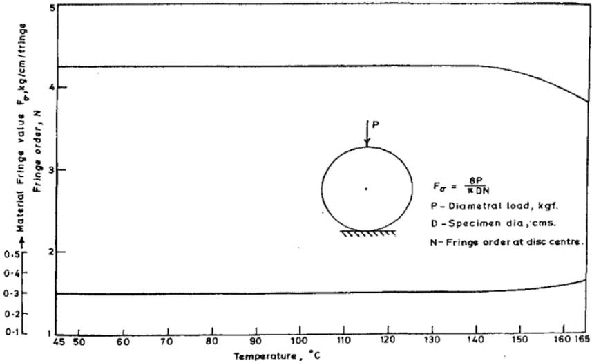
FIG. 5. Variation of material fringe value/order with temperature.
