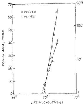
Fig. 3. Determination of pitting life in experiment 4.
