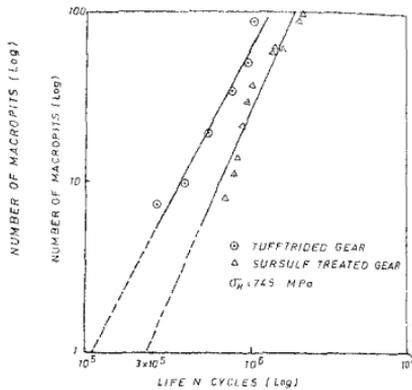
Fig. 4. Relation between number of pits and number of cycles run.
