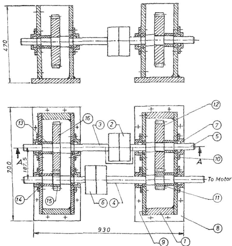
Fig. 1. Gear test rig assembly.
