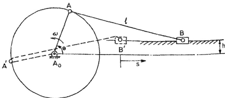
FIG. 7. Off-set slider crank.
