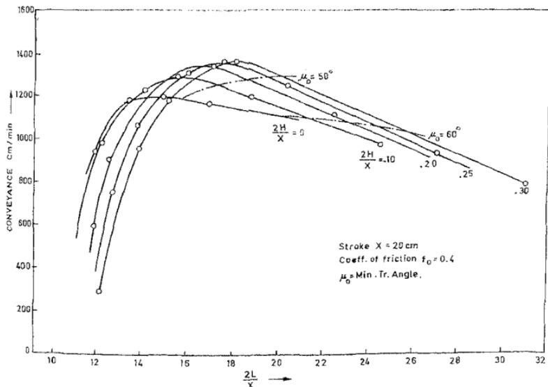
FIG. 8. Optimal conveyance with slider-crank mechanisms
