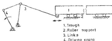
FIG. 1. Constant load-pressure type oscillatory conveyor.
