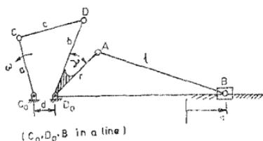
FIG. 10. Slider-crank prefixed with a double crank.
