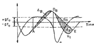
FIG. 3. Velocity and acceleration curves with backward slip.
