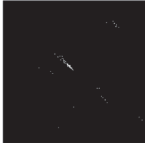
Figure 7: Multilayer model: Wind direction measurement by tracing the peak in the correlation maps data cube.
