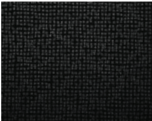
Figure 15: A sample spot pattern image captured by the SHWS camera with the phase plate in the beam path.
