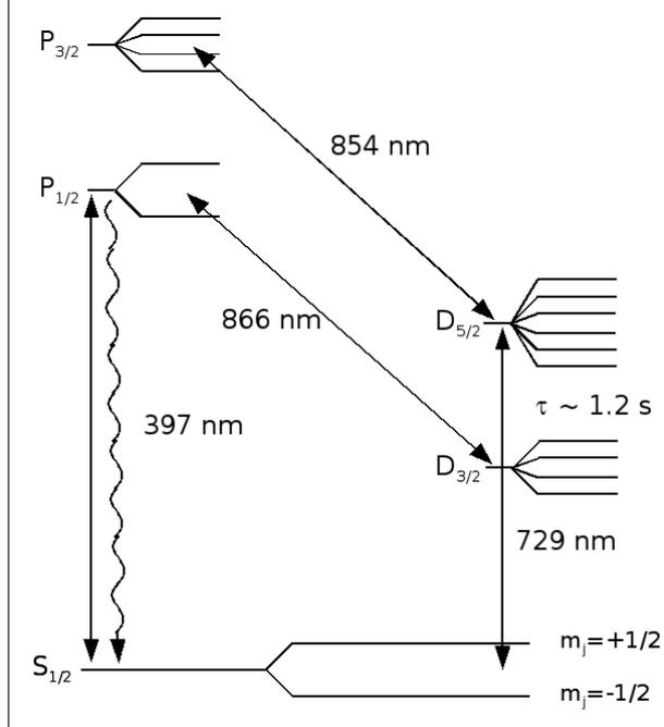
Figure 2: Sideband cooling of a  $^{40}\text{Ca}^+$  ion. The level scheme shows only the most important levels of the ion and of a single motional mode described by a harmonic oscillation with frequency  $\omega_{\text{trap}}$ . Furthermore, it is assumed that the excitation on the  $D_{5/2} \leftrightarrow P_{3/2}$  and the subsequent decay do not change the motional state which is only justified in the Lamb-Dicke regime.
