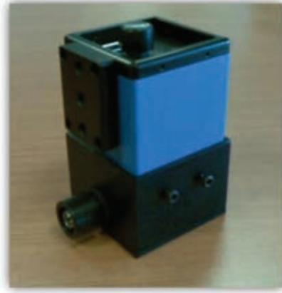
**Figure 6:** Packaged handheld digital holographic microscopy system.<sup>25</sup>
