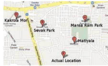
Figure 4: Snapshot of received CBS location messages at a given location. Marker E depicts the current location of the phone and markers A-D presents the four CBS location messages received during phone's stay at E .
