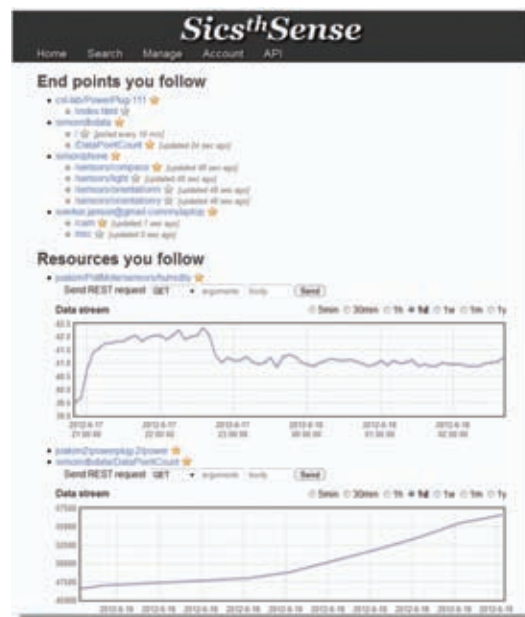
Figure 9: SicsthSense offers a centralized place to manage and share RESTful resources, gather and visualize data, and script actuation.
