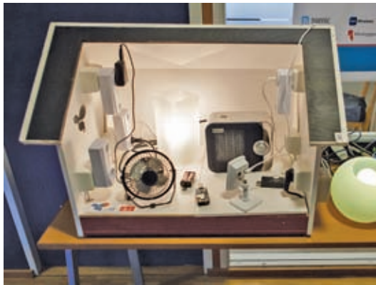
Figure 13: A small scale model of a Smart House based on the architecture shown in Figure 12.
