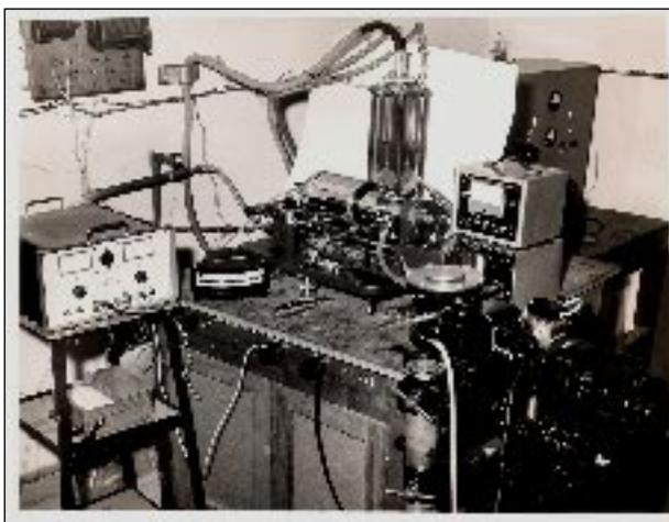
Figure 17: A high temperature furnace for Nonius-Enraf CAD-4 diffractometer up to 500 °C.
