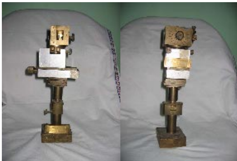
Figure 2: Two perpendicular views of the Frank's optics system fabricated in the physics workshop for focusing X-rays from a rotating anode X-ray generator. X-rays get reflected by two nickel coated mirrors mounted in horizontal and vertical planes, respectively. The system shown is for the vertical mirror. A similar system designed for the horizontal mirror is not shown. The optical system was used for collecting X-ray diffraction data on crystals of PhMV and SeMV. The cradle for housing the mirror has been removed for clarity.
