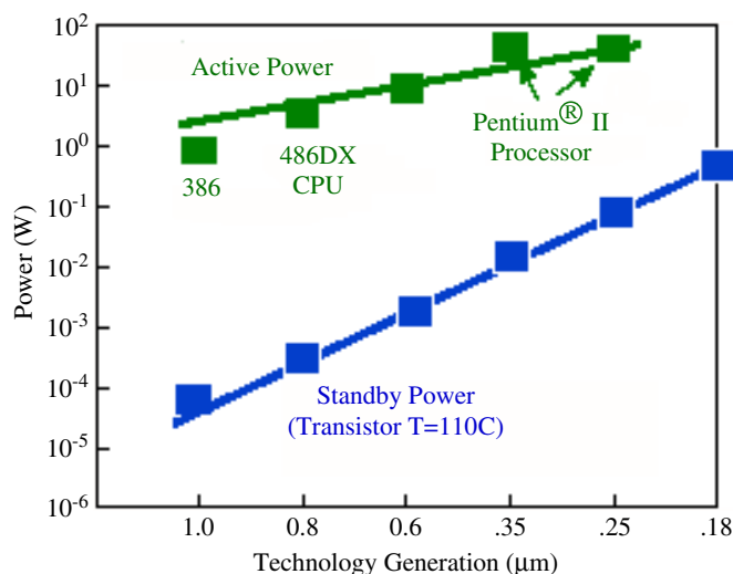
Figure 13: Power dissipation trends with technology scaling [5].
