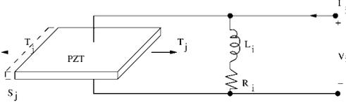
FIG. 2. Resonantly shunted piezoelectric.
