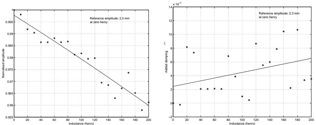
Fig. 7. Response of beam with PZT (inductive shunted).
