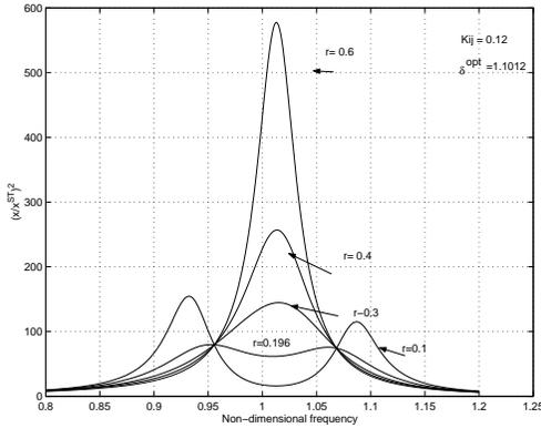
FIG. 4. Response of 1-DOF system containing LRC ( $\delta^{opt} = 1.1012$ ).
