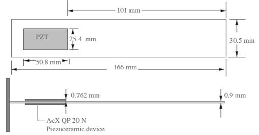
FIG. 5. Beam with PZT.
