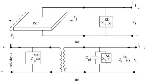
FIG. 1. (a) Physical model of uniaxial shunted piezoelectric and its (b) network analog.
