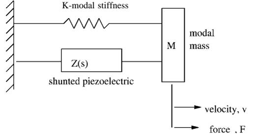
FIG. 3. Single-degree-of-freedom of system model with shunted piezoelectric element in parallel with the system modal mass.
