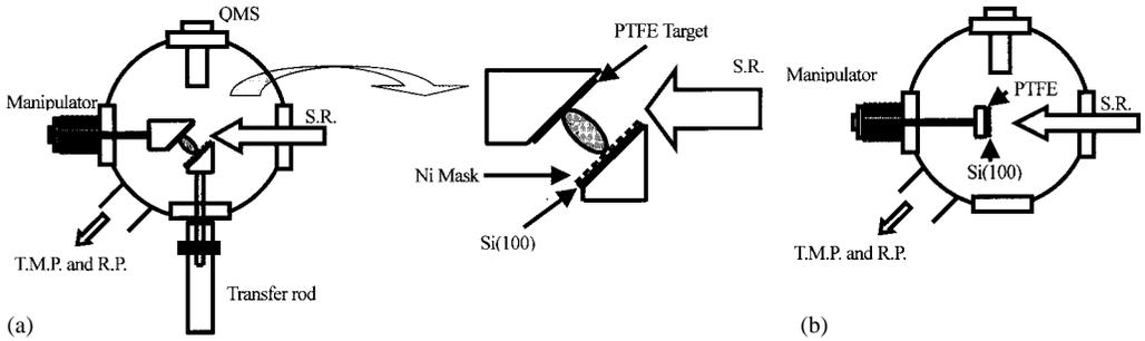
FIG. 1. Experimental set-up for (a) deposition and (b) etching.
