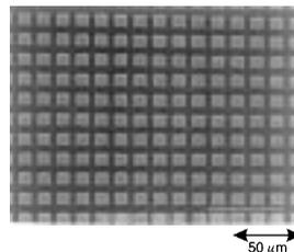
FIG. 2. SEM images of selected deposition of PTFE.
