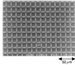
FIG. 3. SEM images of etched surface of PTFE film.
