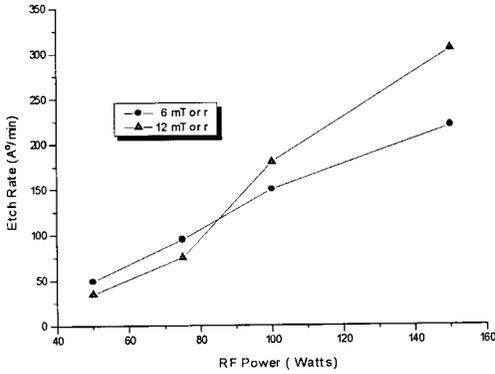
FIG. 1. Variation of SiO<sub>2</sub> etch rate (Å/min) w.r.t. RF power (watts) at two different process pressures at 30 sccm CHF<sub>3</sub> + 5 sccm Ar gas flow rate.
