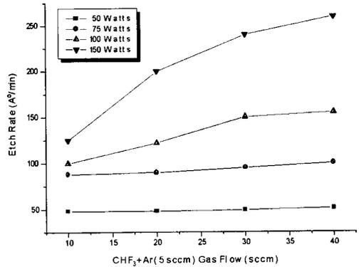
FIG. 2. Variation of SiO<sub>2</sub> etch rate (Å/min) w.r.t. CHF<sub>3</sub> gas flow rate in 5 sccm Ar at different RF power (watts) levels at 6 mtorr process pressure.
