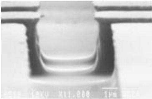
FIG. 4. Etched profile in silicon using  $\text{SF}_6/\text{O}_2/\text{CHF}_3$  gas mixtures.
