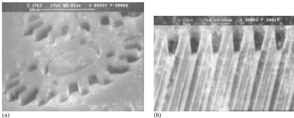
FIG. 3 Microstructures etched in  $\text{SiO}_2$  by RIE: (a) microgears and (b) grating pattern.
