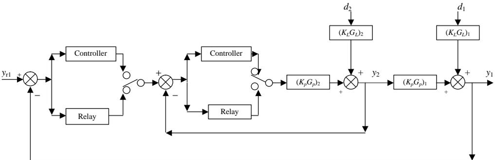
FIG. 1. Relay feedback tuning of cascade control system.
