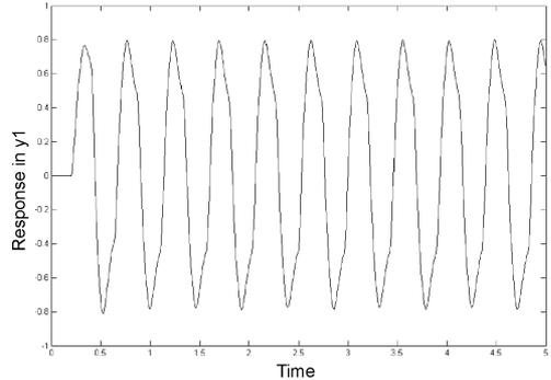
FIG. 3. Response in  $y_1$  for symmetric relay in outer loop (with inner loop on PI settings).
