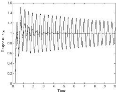
FIG. 4. Servo response in  $y_1$  using PID controller for outer loop and PI for inner loop for the first example. Outer oscillatory response – Hang *et al.* method; Inner solid–proposed method-1; Inner dash–proposed method-2.
