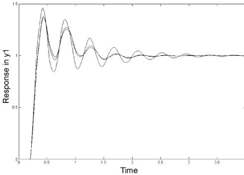
FIG. 6. Servo response in  $y_1$  using PID controller for outer loop and PI for inner loop for the second example. Inner solid—proposed method-1; Inner dash—proposed method-2.
