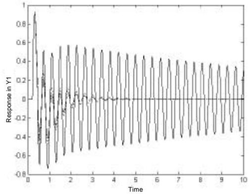
FIG. 5. Regulatory response in  $y_1$  for a disturbance in inner loop. PID controller for outer loop and PI for inner loop, for the first example. Inner solid–proposed method-1; Inner dash–proposed method-2.
