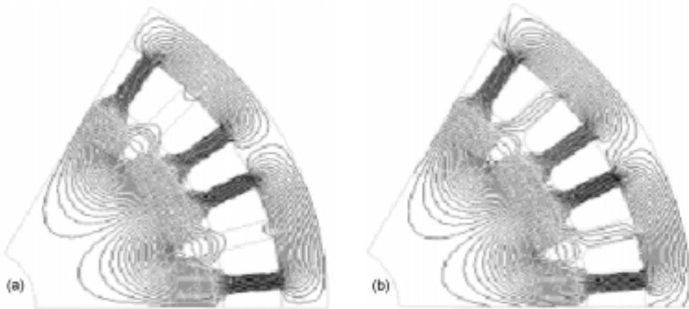
FIG. 5. Flux lines for (a) minimum, and (b) maximum cogging torque positions.
