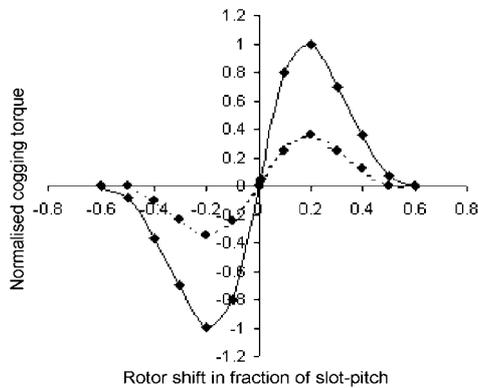
FIG. 3. Plot of normalized cogging torque against rotor shift. —◆— Uniform air-gap; ---◆--- Nonuniform air gap.
