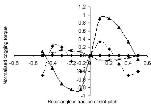
FIG. 6. Cogging torque for different skewing angles and for optimized PM width. —◆— Full skew; - - \* - - Fractional skew; —▲— Original condition; ---◆--- With optimized width.
