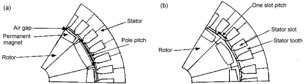
FIG. 2(a). Permanent magnet with uniform air-gap. (b) Permanent magnet with nonuniform (bread loaf) air gap.
