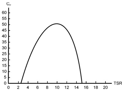
FIG. 1. A typical  $C_p$  curve for wind generator.
