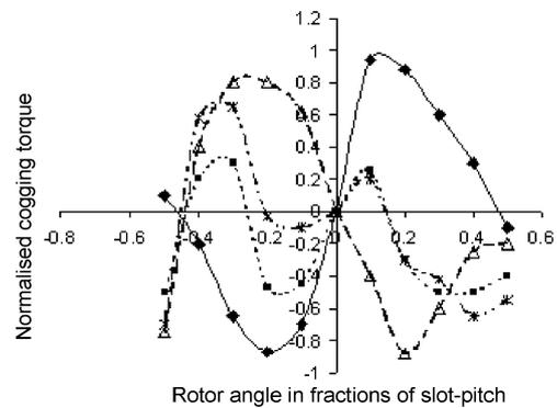
FIG. 4. Cogging torque for different PM width. —◆— Original PM width; ---■--- 0.9 of PM width; - - \* - - 0.88 of PM width; . . Δ . . 0.85 of PM width.
