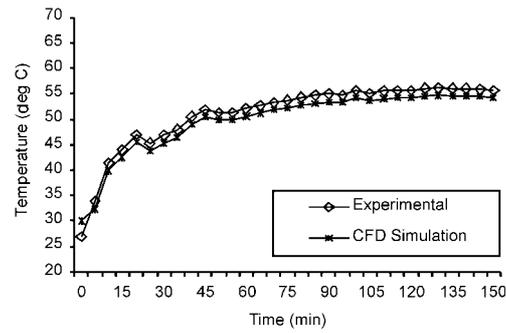
FIG. 10. Comparison of experimental and CFD simulation results for foodstuff (9).
