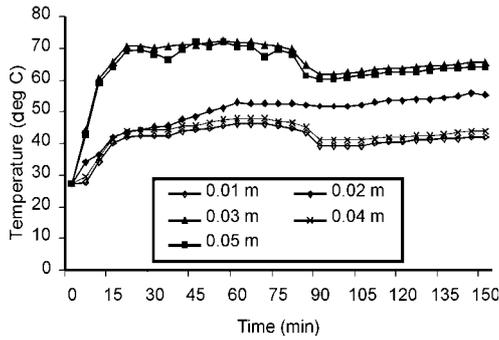
FIG. 5. Temperature variation of foodstuff with time for different coil diameters.
