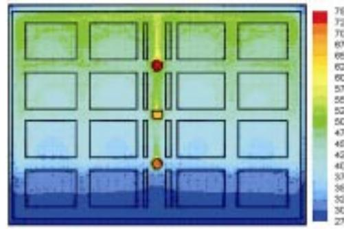
FIG. 6. Temperature distribution inside the display cabinet—middle coil location.
