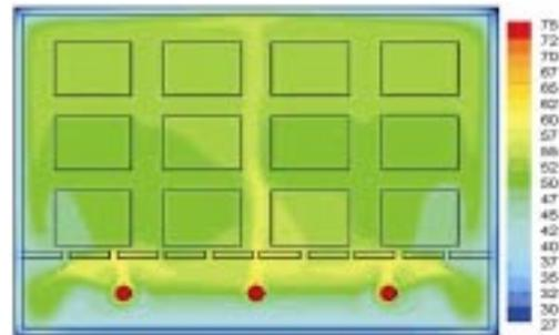
FIG. 4. Temperature distribution inside the display cabinet—bottom coil location.
