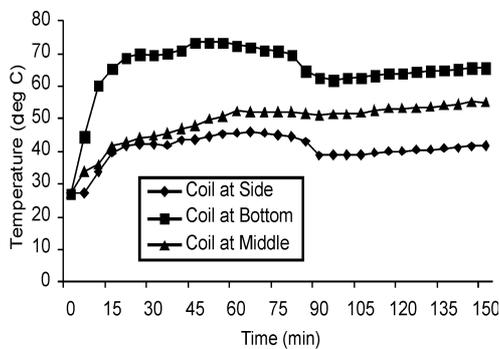
FIG. 7. Temperature variation of foodstuff(10) with time for different positions.
