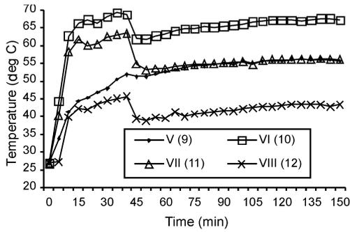
FIG. 9. Temperature variation of foodstuff with time for the bottom row-experimental.
