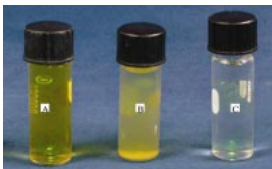
FIG. 3. Impact of HRP on the removal of direct yellow-12 dye. A: Direct yellow-12 dye; B: Reaction mixture; C: End result.
