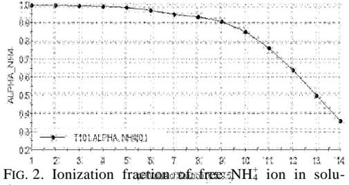
FIG. 2. Ionization fraction of free  $NH_4^+$  ion in solutions.
