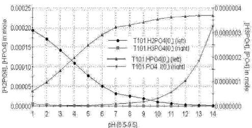
FIG. 3. Variations of concentration of different phosphate ions with pH in solution.
