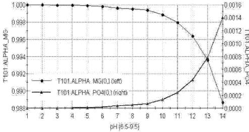
FIG. 1. Ionization fraction of free  $Mg^{2+}$  and  $PO_4^{3-}$  ions in solutions.
