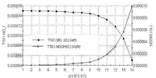
FIG. 4. Variations of concentration of different magnesium ions with pH in solution.
