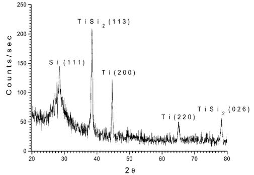
FIG. 2. GIXRD spectra of Au ion (95 MeV)-irradiated Ti/Si specimen.
