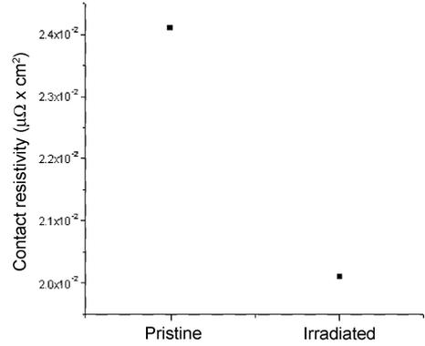
FIG. 4. Resistivity plot of Ti-Si samples before and after Au ion (95 MeV) irradiation.
