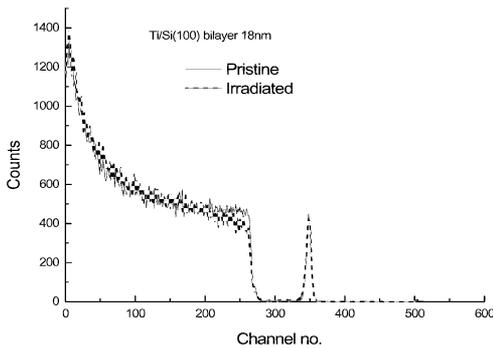
FIG. 1. RBS spectra of pristine and Au ion (95 MeV)-irradiated Ti/Si specimen.
