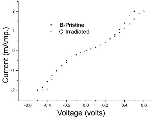
FIG. 3. I-V characteristics of pristine and Au ion (95 MeV)-irradiated Ti-Si specimen.
