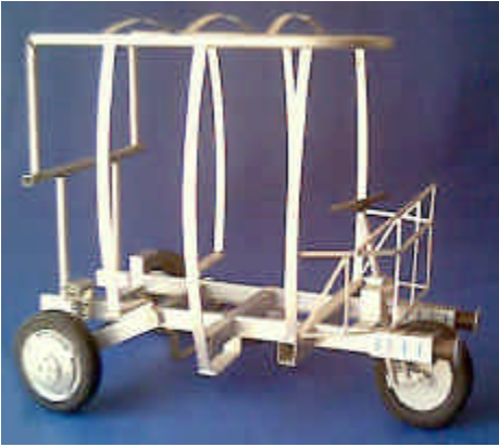
FIG. 10. Chassis with crash bumpers for Design 2.
