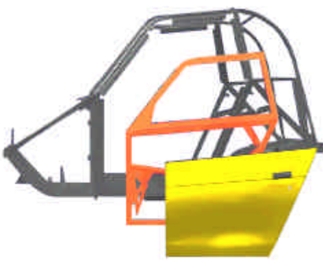
FIG. 12. Three levels of safety–dent-proof body panels, side impact beams and a steel space frame.
