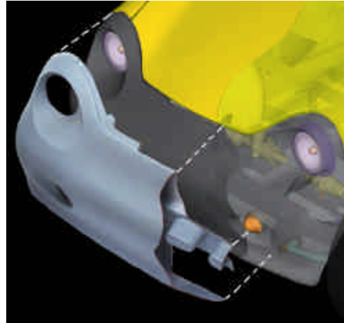
FIG. 13. Bumpers: designed with energy-absorbent crush cones.
