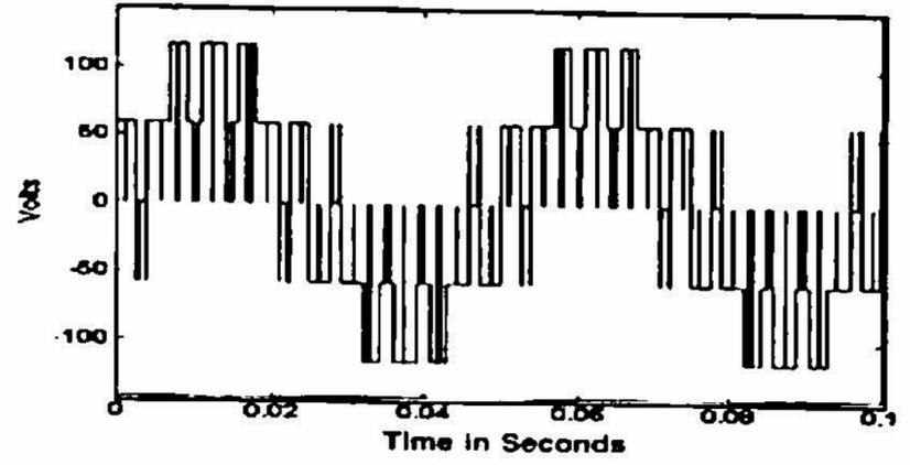
Fig. 2h. Simulated waveform of the phase voltage  $v_{A2N}$  in 2-level inversion mode which is on the verge of changing over to 3-level inversion mode (corresponding to the condition of Fig. 2b).
