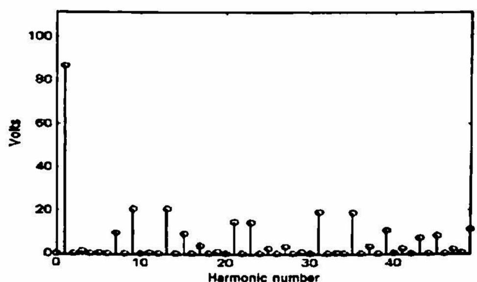
Fig. 2f. The harmonic spectrum of the motor phase voltage  $v_m$  at 3-level mode of operation on the verge of changing over to 2-level operation (refer Fig. 2c).
