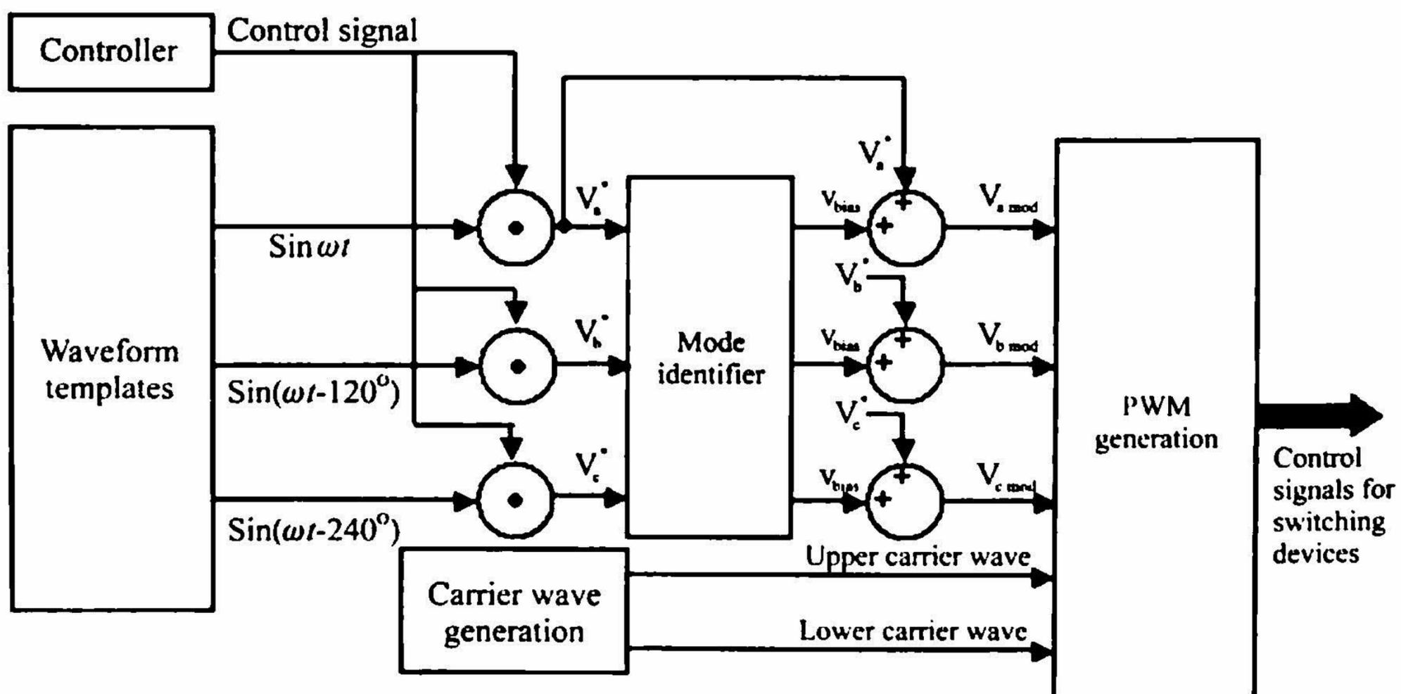
Fig. 3. Implementation of the modified SPWM scheme for the proposed 3-level inverter ( $v_{bias} = 0$  in 2-level inversion mode and  $v_{bias} =$  peak value of the lower carrier wave in 3-level inversion mode).
