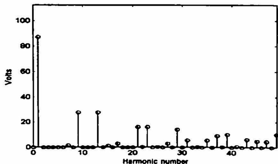
Fig. 2e. The harmonic spectrum of the motor phase voltage  $v_m$  at 2-level mode of operation on the verge of changing over to 3-level operation (refer Fig. 2b).
