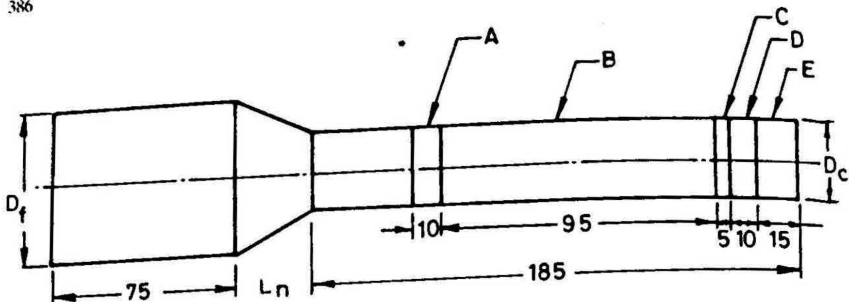
FIG. 1. Details showing location of test specimens in the test casting taken for various tests.
