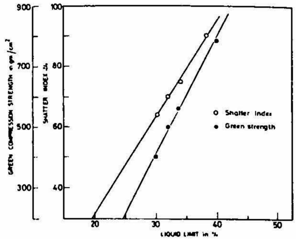
FIG. 4 Relationship of liquid limit with green compression strength and shatter index.
