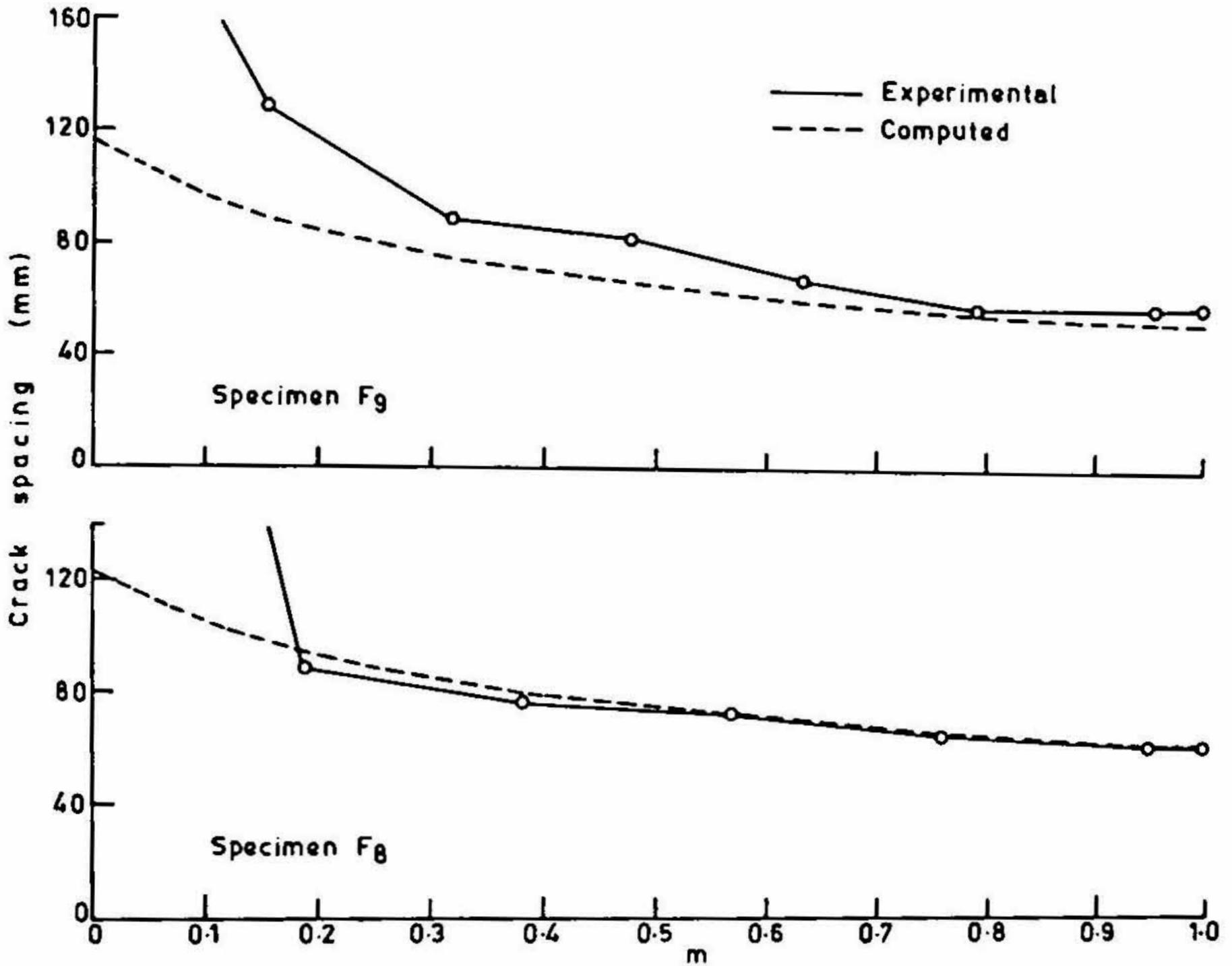
FIG. 3. Variation of crack spacing against the factors 'm' for specimens F8 and F9.
