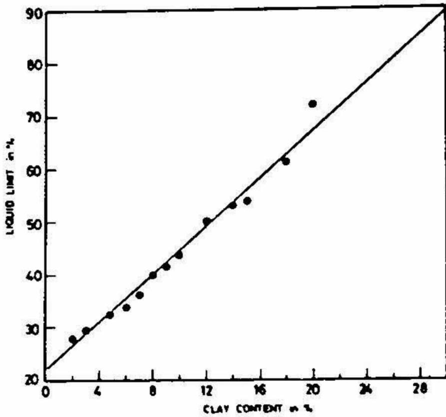
FIG. 3 Relationship between clay content and liquid limit
