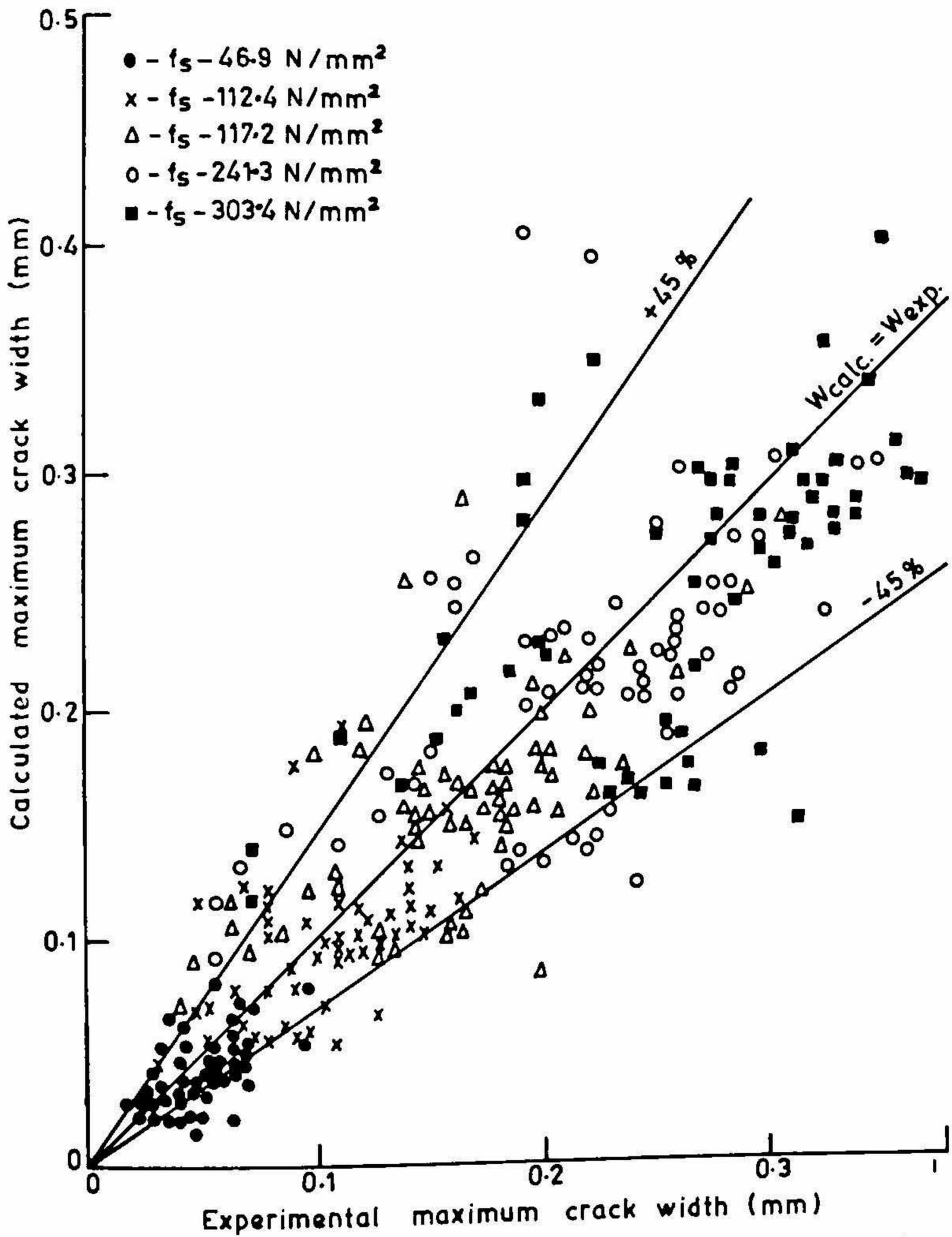
FIG. 1. Comparison of calculated crackwidths with the experimental crackwidths of Base *et al*<sup>4</sup>.
