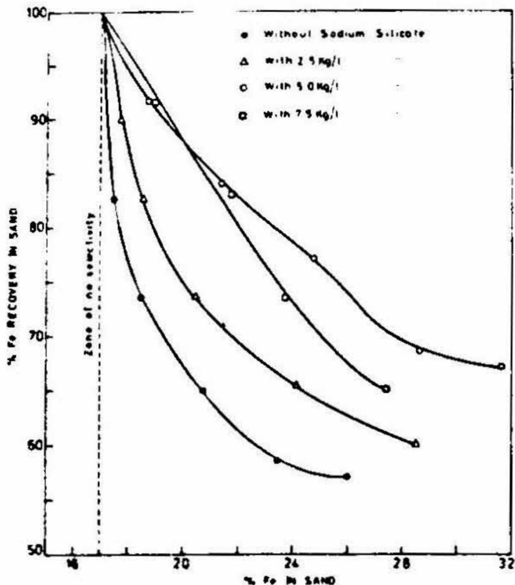
FIG. 2 Selective flocculation studies on mixtures of pyrite and quartz with starch xanthate (0.2 g) as a function of sodium silicate.
