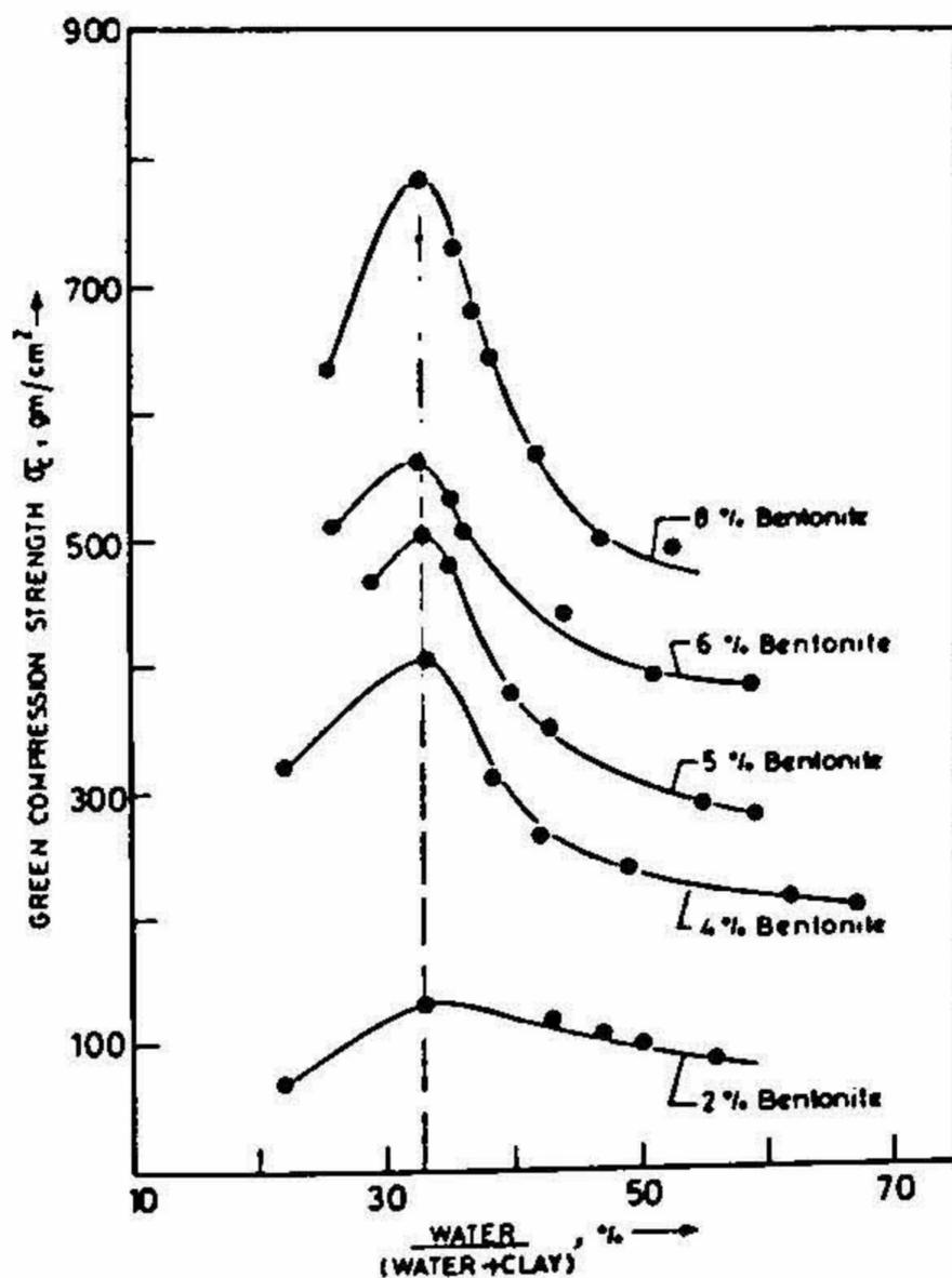
FIG. 1. Influence of water: clay ratio and bentonite content on green compression strength.
