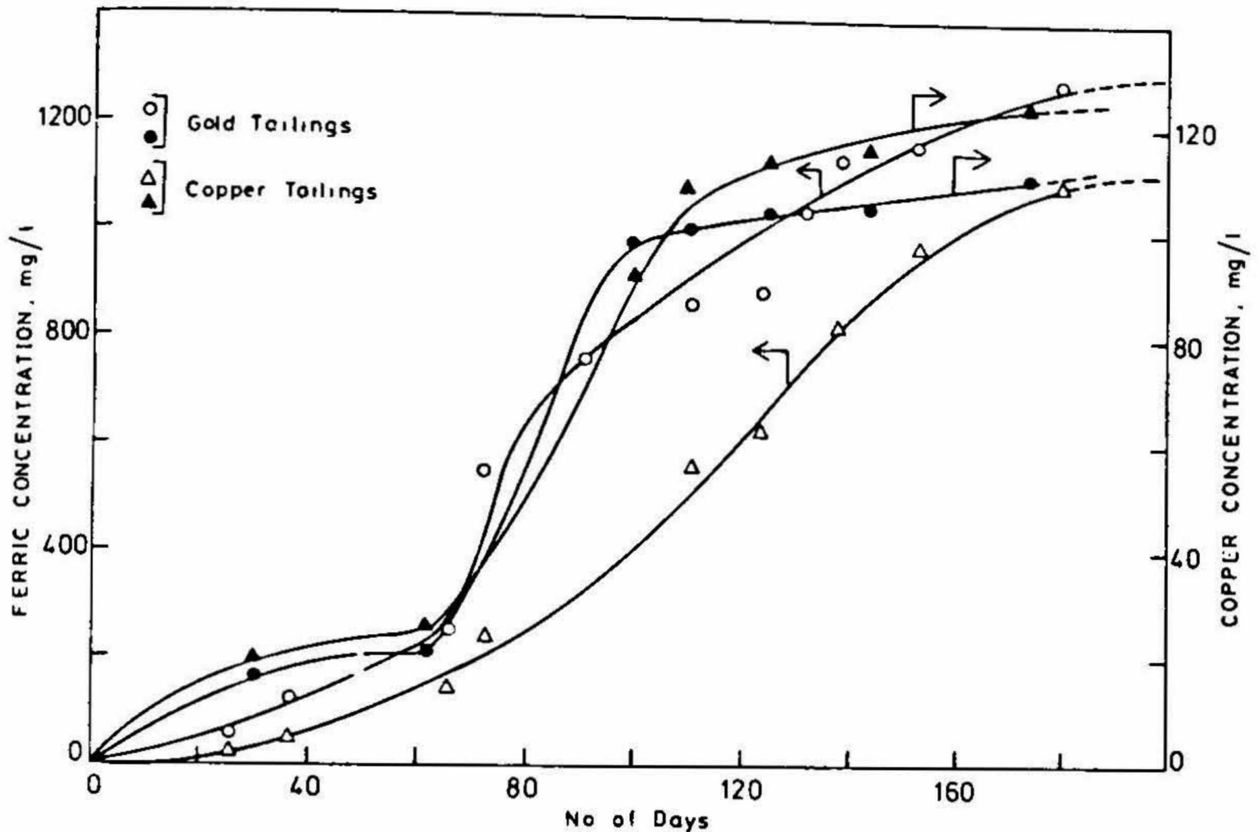
FIG. 1. Variations of ferric ion concentration and copper ion concentration with time in environmental column leaching of copper and gold tailings in the presence of bacteria.
