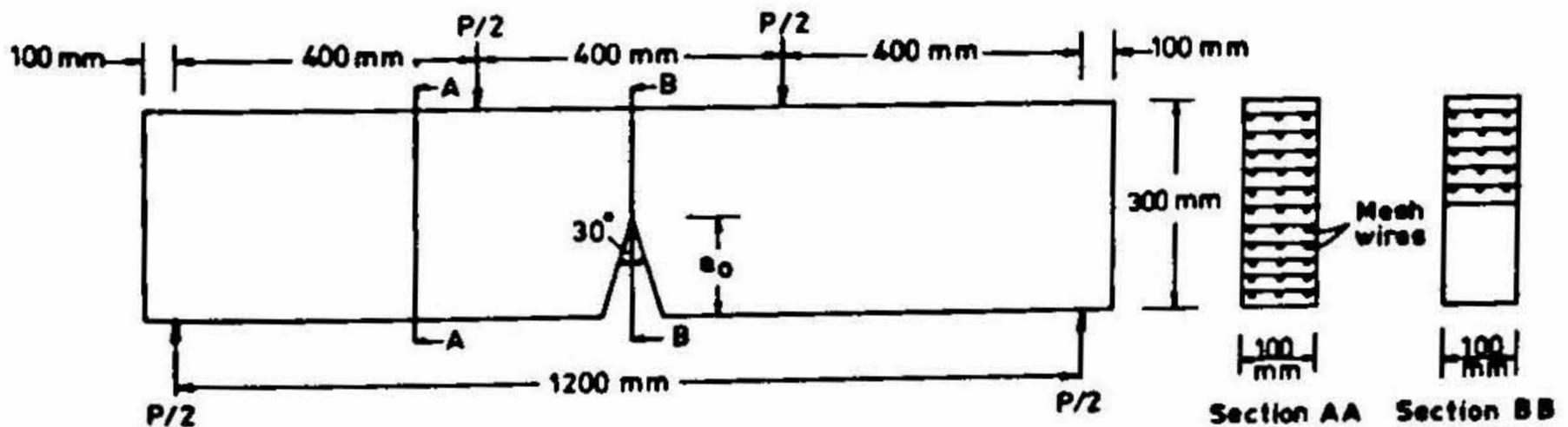
FIG. 4. Dimensions of ferrocement notched beam specimen.
