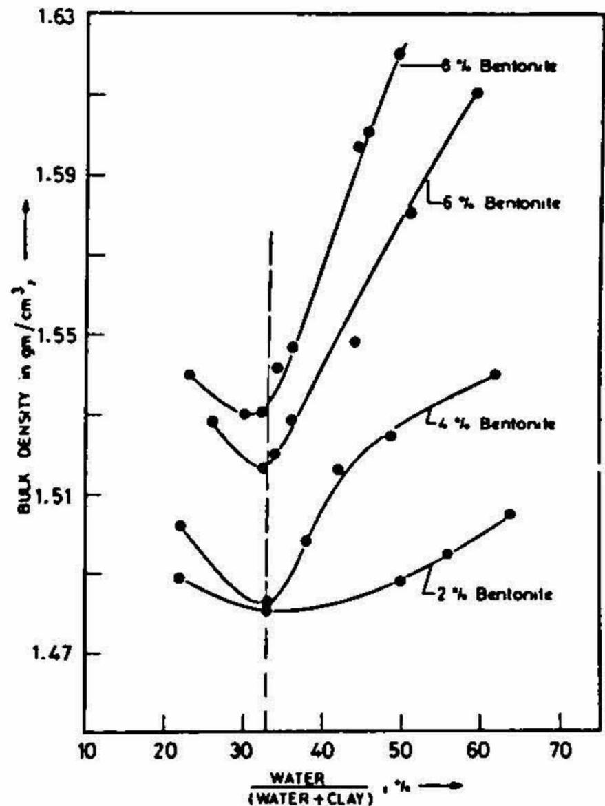
FIG. 2. Influence of water: clay ratio and bentonite content on bulk density.
