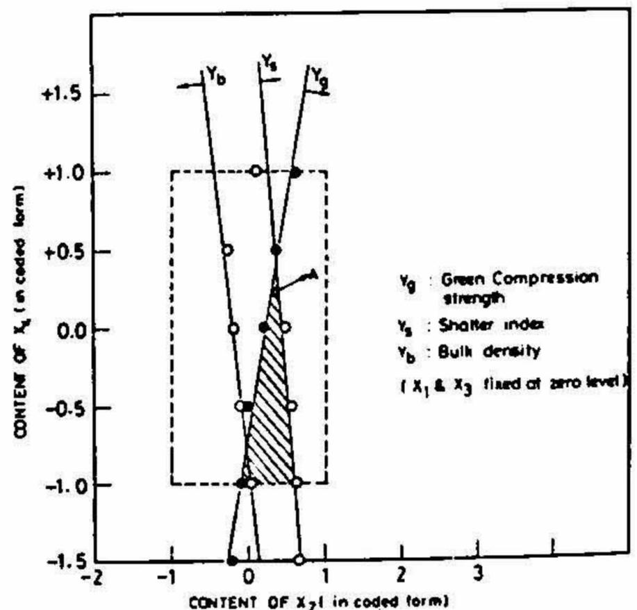
FIG. 6. Nomogram for optimising sand composition (Additive: Starch).
