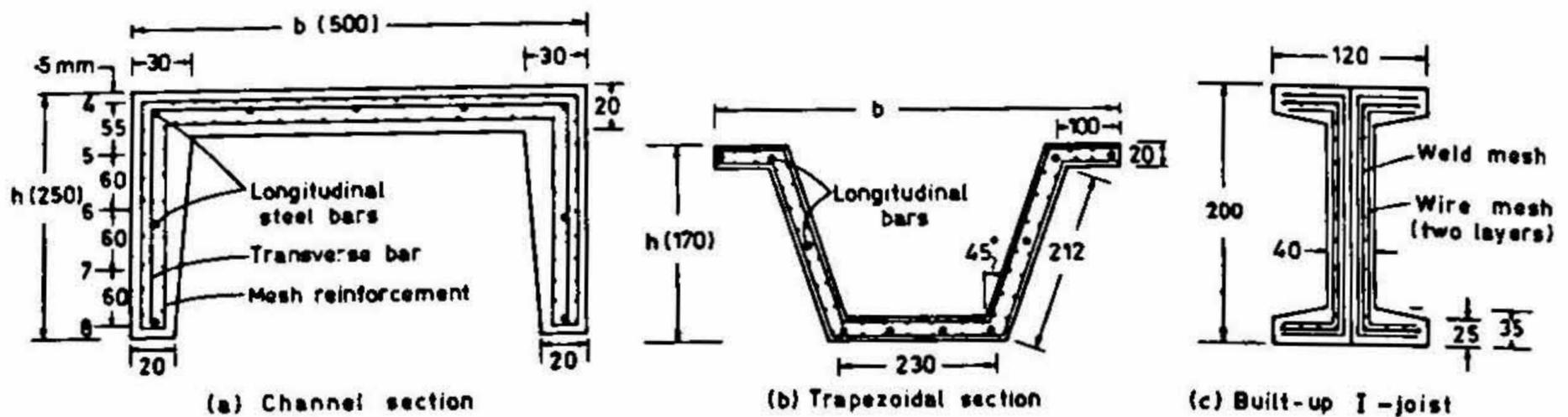
FIG. 2. Details of cross-sections of ferrocement flexural members (in mm).
