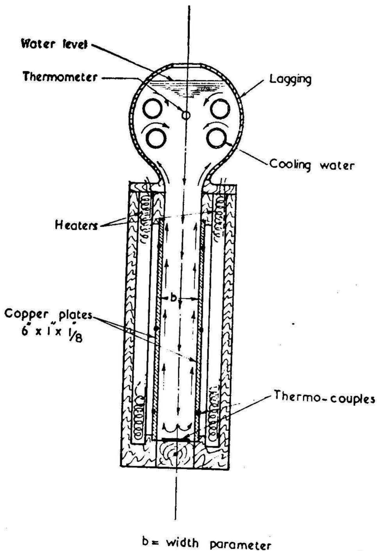
FIG. 1. Apparatus for studying heat transfer by convection from parallel plates to fluids.
