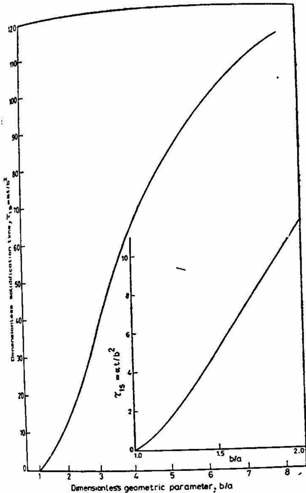
Fig. 5. Solidification time of hollow plates (LM6 alloy)—generalised.
