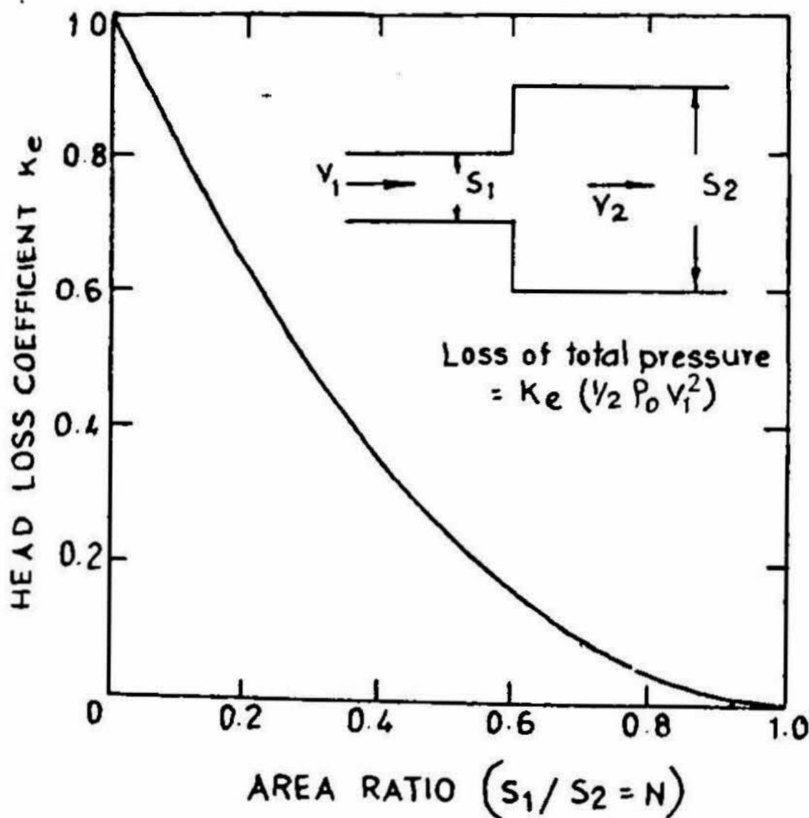
FIG. 3. Head loss coefficient  $K_e$  vs area ratio at sudden expansion, — experimental  $K_e = (1 - N)$  from references 10 and 11.
