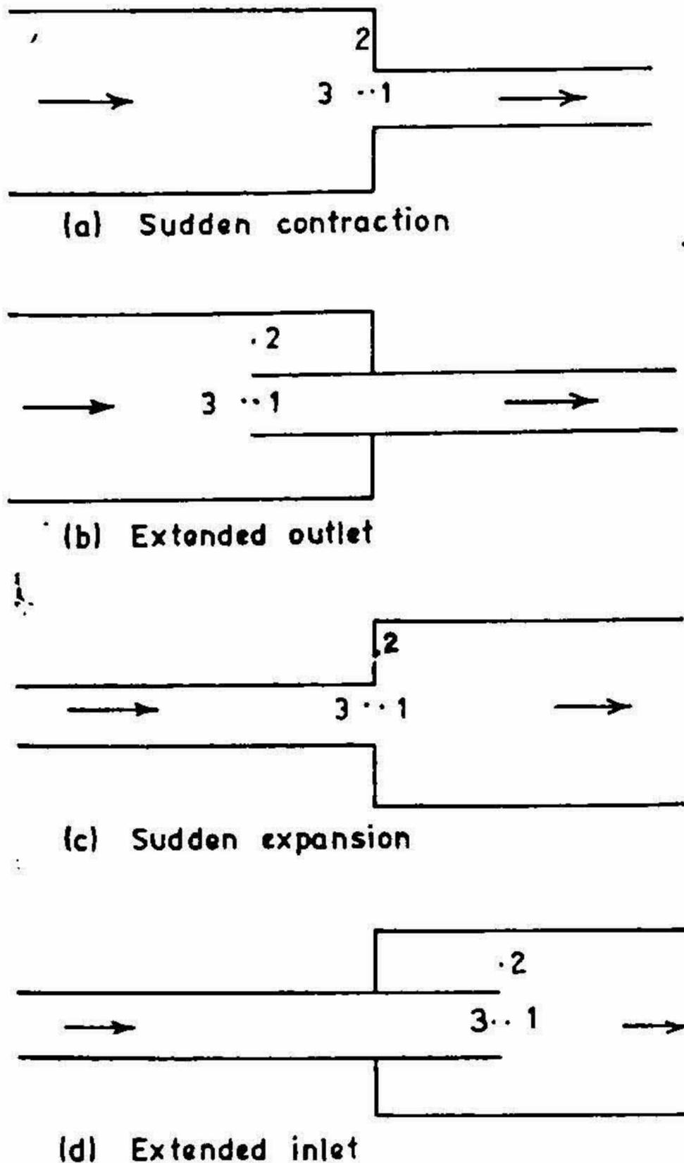
FIG. 1. Muffler elements with abrupt area changes.
