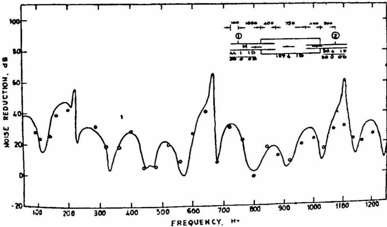
FIG. 9. Noise reduction vs frequency for a muffler with extended inlet and extended outlet with flow.  $M = 0.06$ . — theoretical; o o experimental.
