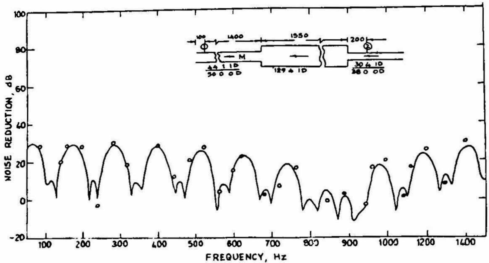
FIG. 6. Noise reduction vs frequency for a simple expansion chamber muffler without flow. — theoretical; o o experimental.
