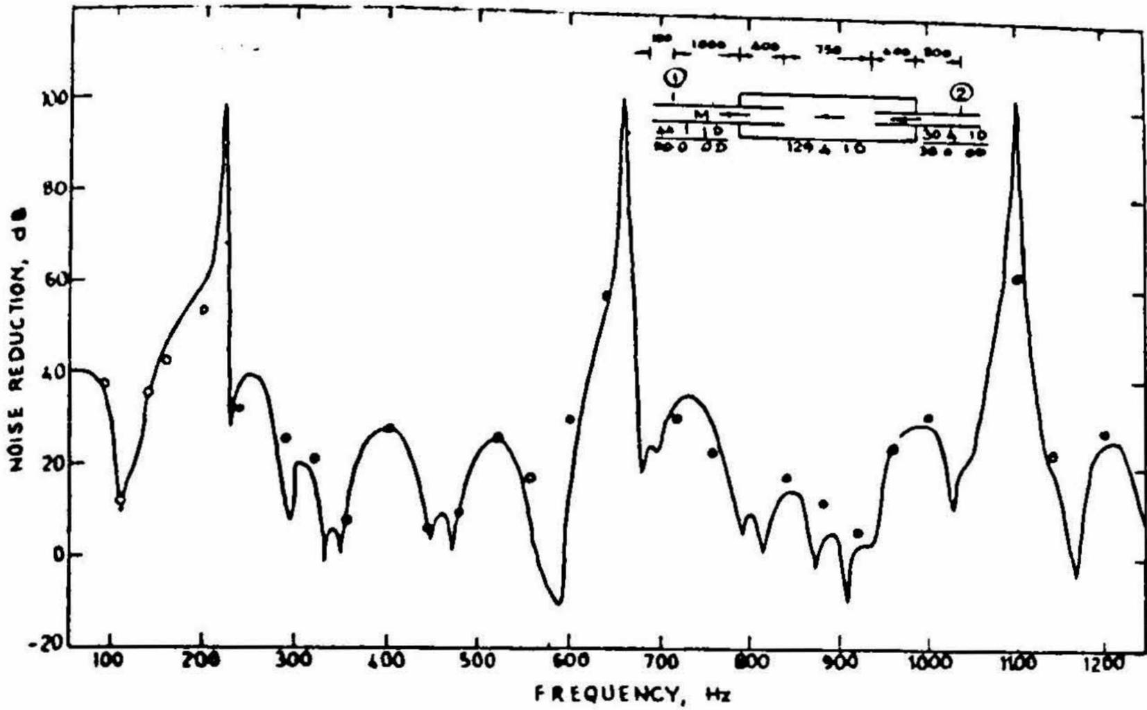
FIG. 8. Noise reduction vs frequency for muffler with extended inlet and extended outlet without flow. — theoretical; o o experimental.
