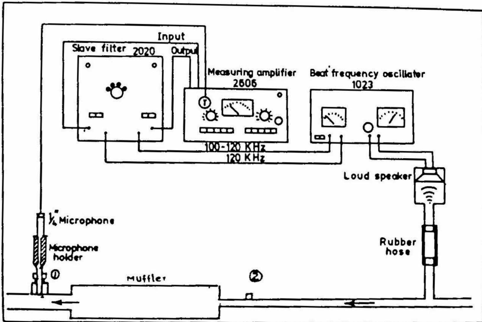
FIG. 5. Schematic arrangement of excitation-cum-measurement system.
