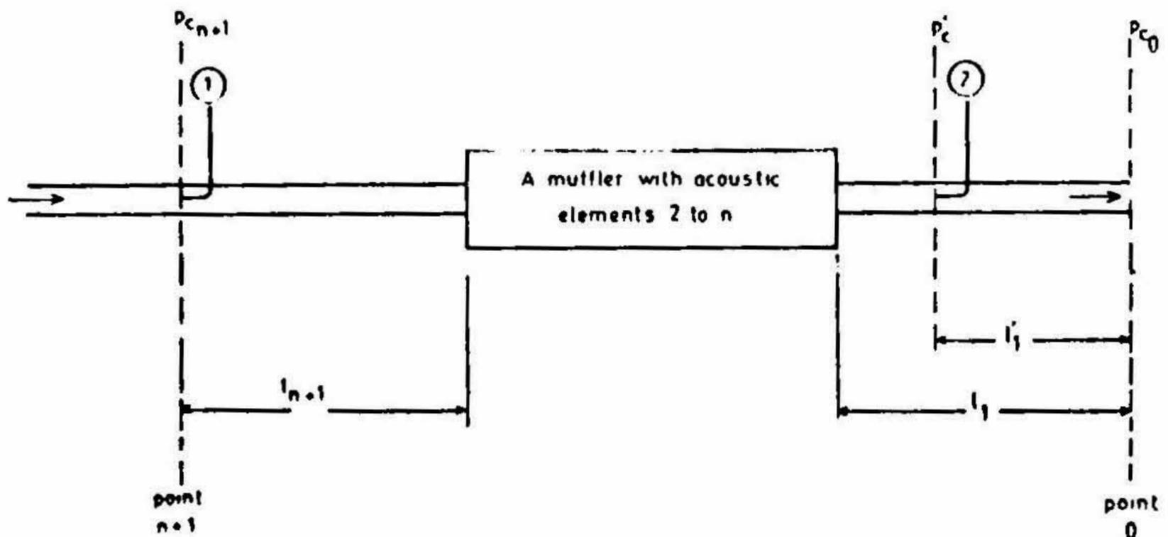
FIG. A-1. Terminology for noise reduction parameter.
