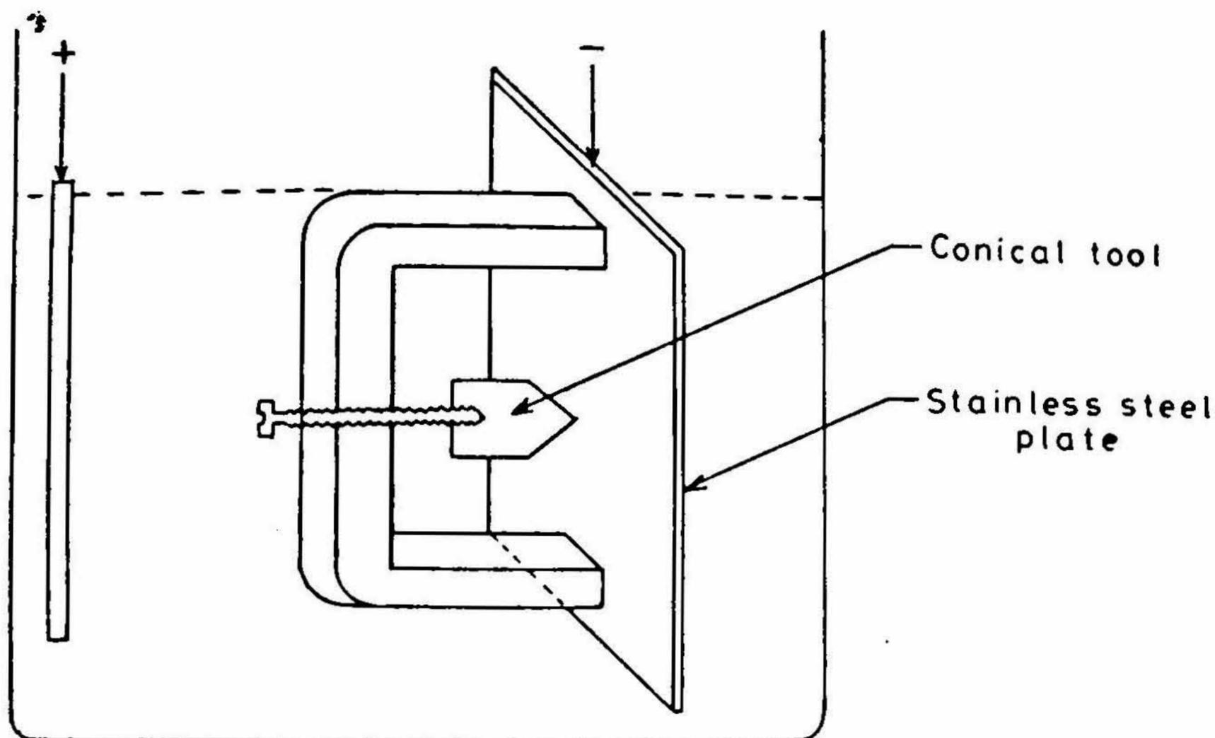
FIG. 2. Schematic diagram of the sample-holder used in the electroforming method.
