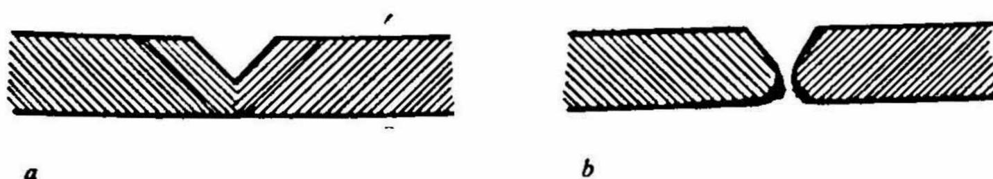
FIG. 3. Results of the laser punching method : (a) before punching ; (b) after punching.
