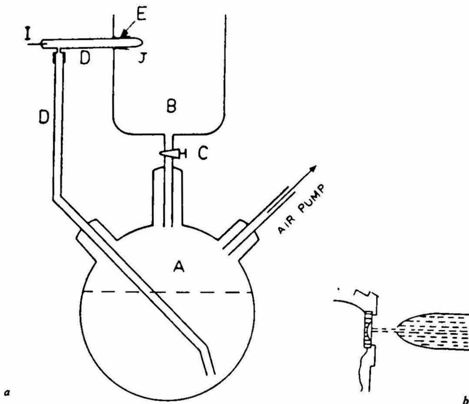
FIG. 7. (a) Schematic diagram of the single Jet polishing unit ; A—Round bottom flask ; B—Sink for collecting the electrolyte ; C—Stop-cock ; D—Glass tube ; E—Standard joint ; I—Platinum wire which acts as a cathode ; J—Jet. (b) Schematic representation of single jet operation.
