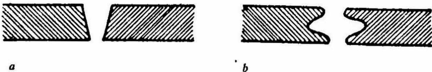
FIG. 1. Photolithographic method : (a) Expected configuration ; (b) Observed configuration.
