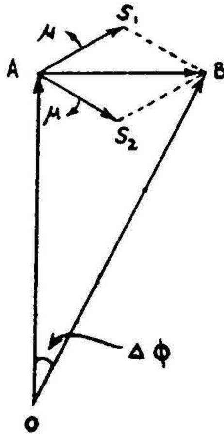
FIG. 2. Vector Diagram of the Armstrong FM System based on the zero frequency carrier concept
