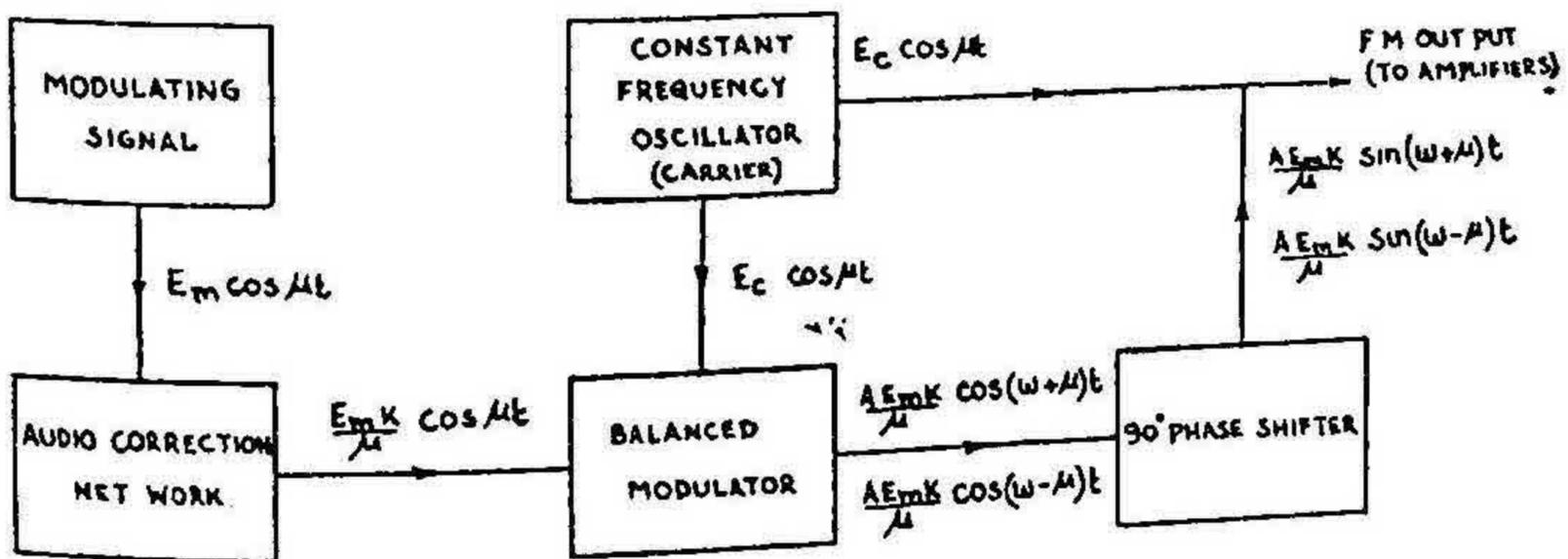
FIG. 1. Armstrong System of Frequency Modulation
