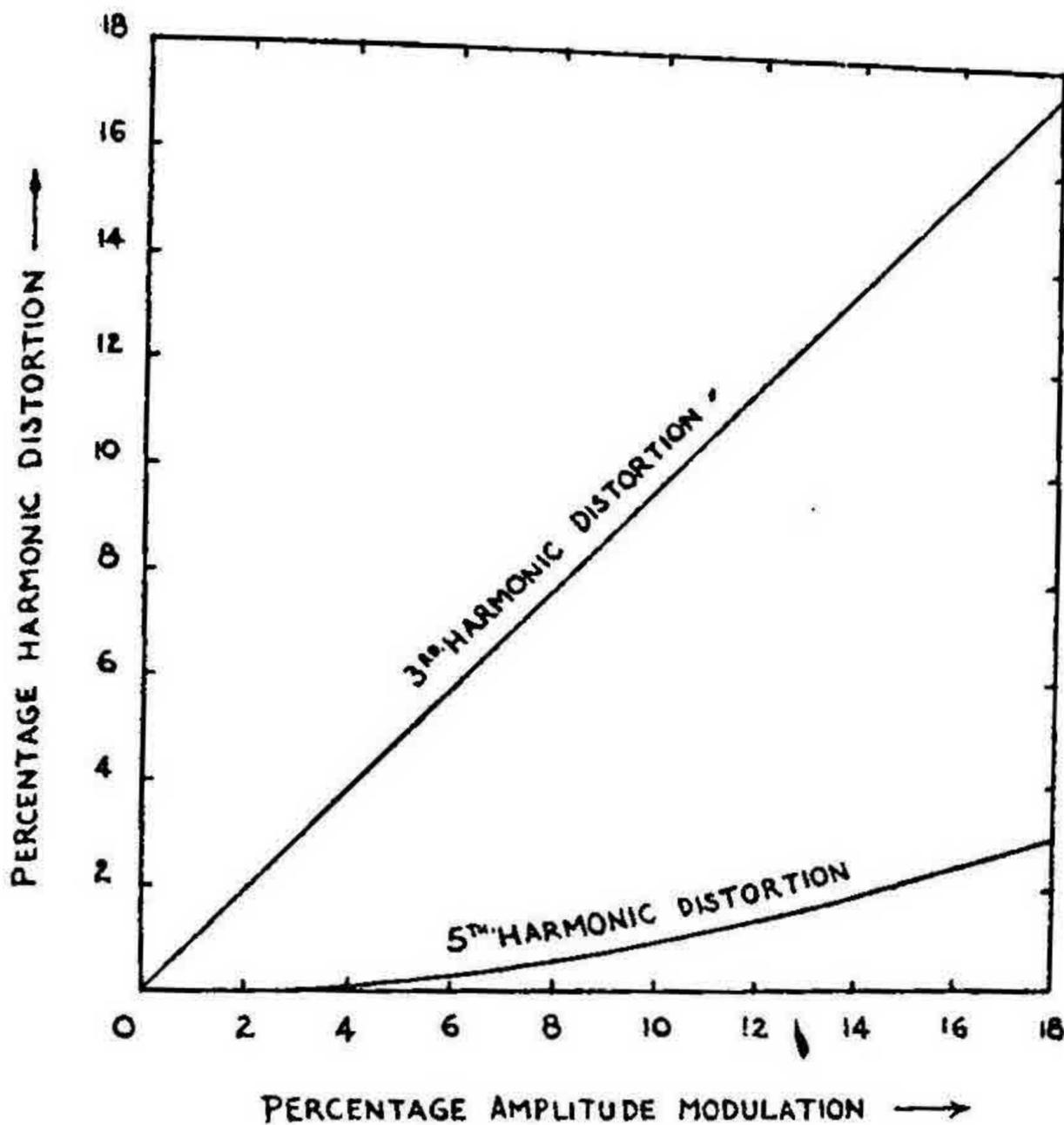
FIG. 5. Percentage of Harmonic Distortion vs. Percentage of Amplitude Modulation
