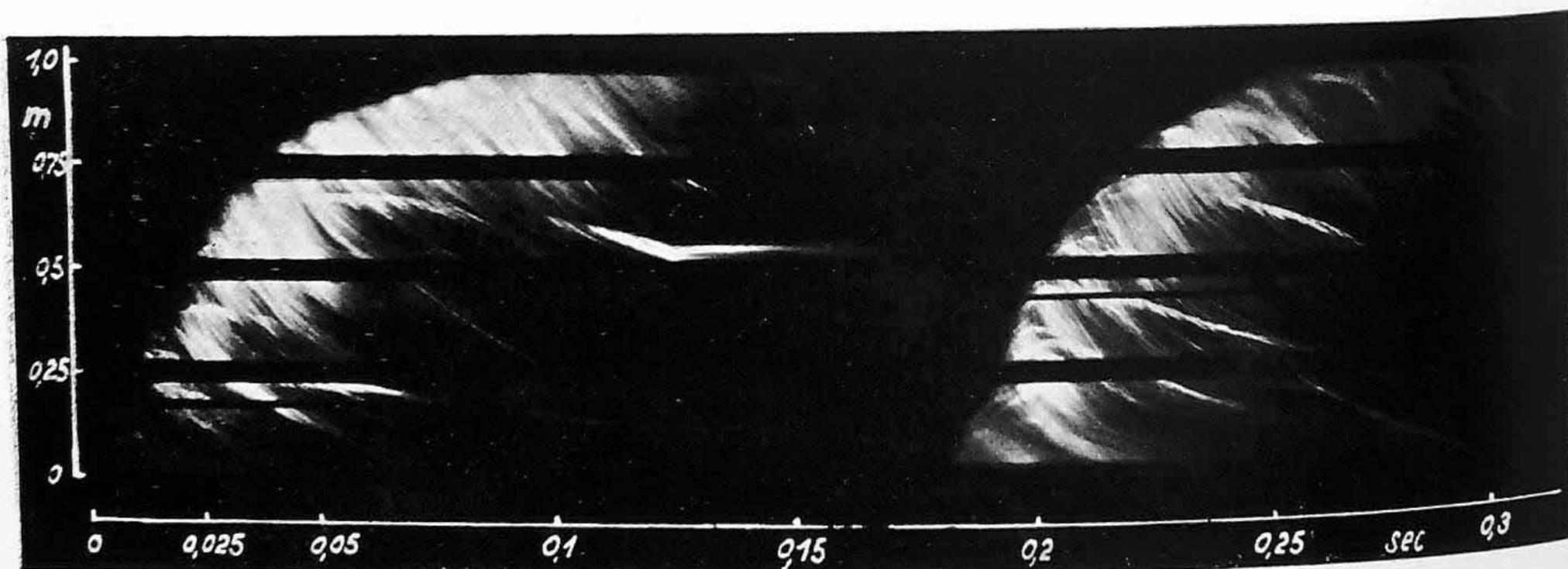
FIG. 53. Combustion of precompressed oscillating propane-air-mixtures  $\lambda=1$  (air pressure 5 ata).
