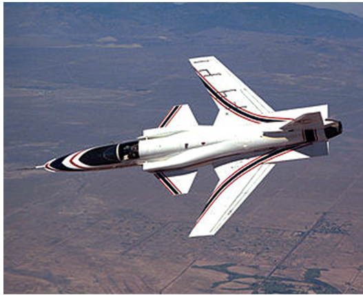
Figure 6: Forward swept wing in X-29 aircraft.
