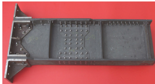
Figure 15: Spar splice joint.
