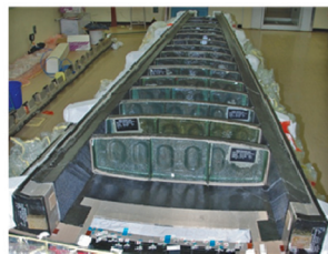
Preform Assembly of Outboard Bottom Skin
