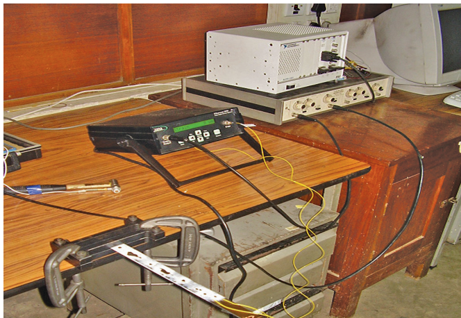
Figure 11: Experimental set up for dynamic response measurement of a cantilever beam made of glass fiber reinforced polymer composite with surface bonded EFPI sensor.
