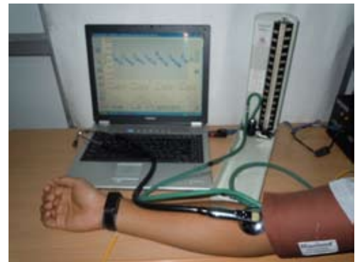
Figure 14: Simultaneous data acquisition from FBGPD and the electronic stethoscope during sphygmomanometry. 53
