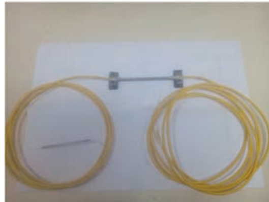
Figure 5: Photograph of the packaged FBG sensor for cementitious mounting.
