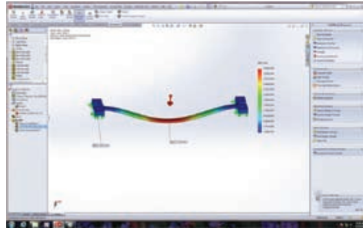
Figure 4: Result of the FE analysis for FBG packing fixture.
