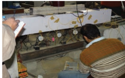
Figure 6: Photograph of RC Beam under test in the laboratory.
