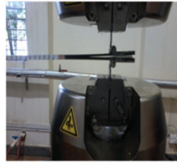
(a) Double cantilever beam (DCB) specimen for Mode I delamination toughness
