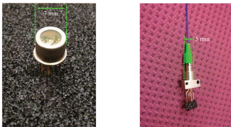
Figure 4: Images of free-space (left) and fiber-coupled (right) Vertical-Cavity Surface-Emitting Lasers (VCSELs), indicating their compactness.
