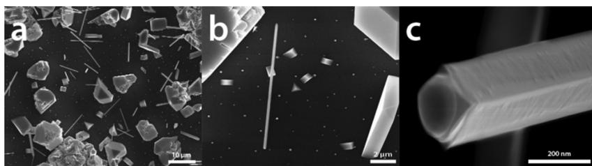
**Figure 4:** (a) Low resolution SEM image of nanowires and microcrystals. (b) Nanowire of SnTe surrounded by Au nanoparticles. (c) High resolution SEM image of the tip of a SnTe nanowire; an alloy can be seen.
