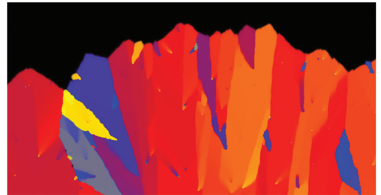
Figure 8: Orientation map from a phase-field model of spherulitic solidification relying on an orientation field. 78,79 The formation of orientation defects at the solid-liquid interface is shown that initiate new grains. Different colors correspond to different crystallographic orientations. Sharp changes in color stand for grain boundaries (coherent dislocation lines), whereas the orientation defects can be interpreted as bundles of dislocations. The liquid domain is black.
