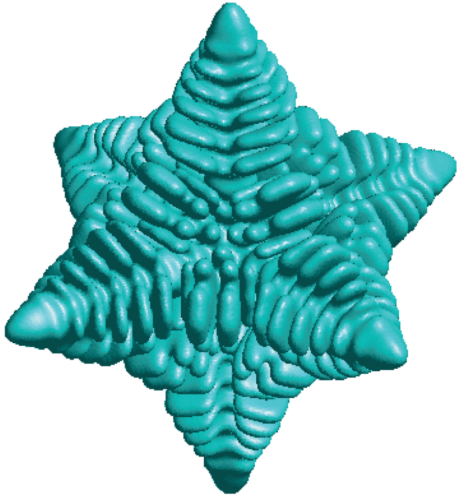
Figure 5: Dendrite simulated with the anisotropic Karma-Rappel model, with an anisotropy of the surface free energy given by Eq. (72) with \varepsilon_4 = 0.00625 , and isotropic (vanishing) kinetics ( \beta(\hat{n}) = 0 ). The dimensionless undercooling is \Delta = 0.1 , that is, the initial and boundary values of u = -0.1 . The simulation is carried out with the multi-scale algorithm described in Ref. 41
