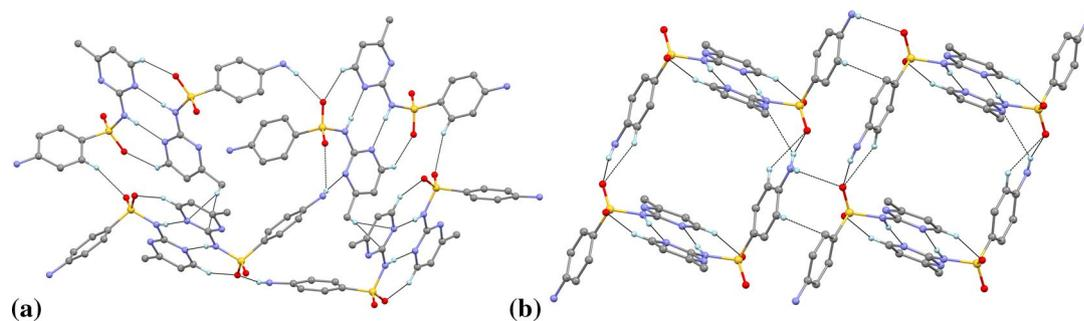
**Figure 18:** Different association of dimeric motifs in **a** form I and **b** form II polymorphs through N-H...O, N-H...N, and C-H...O interactions.
