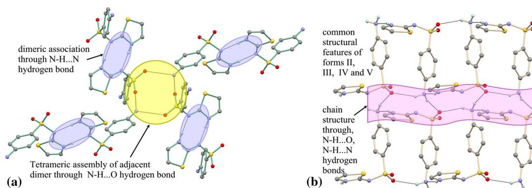
**Figure 27:** Association of sulfathiazole molecules in **a** form I (dimeric motif) and **b** form III crystals (catemeric motif).
