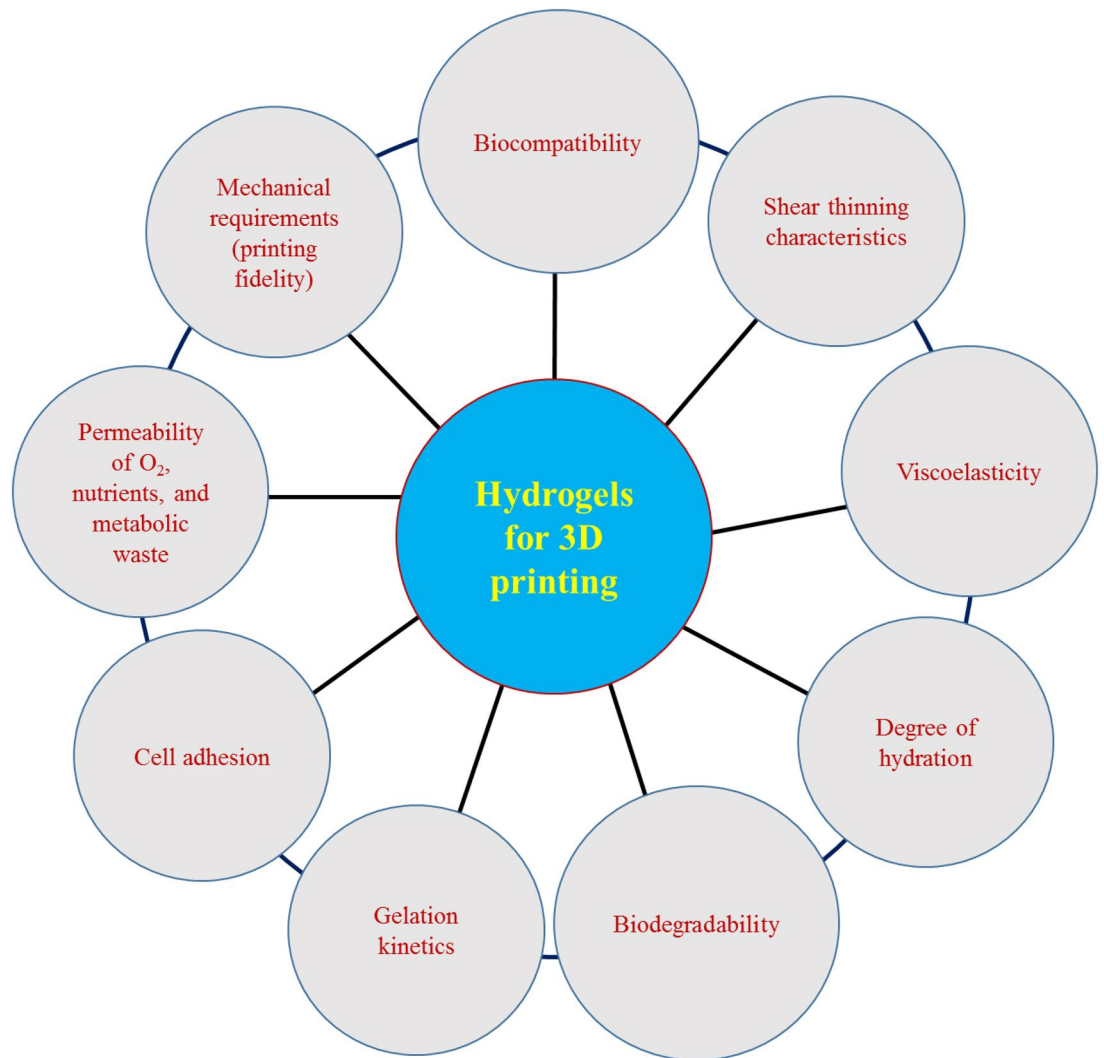
Figure 4: Schematic of the spectrum of properties required for ideal bioink formulation in 3D bioprinting 19, 116
