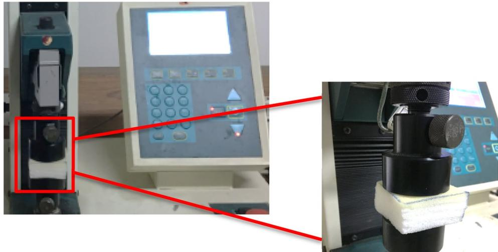
**Figure 1:** Compression test setup.
