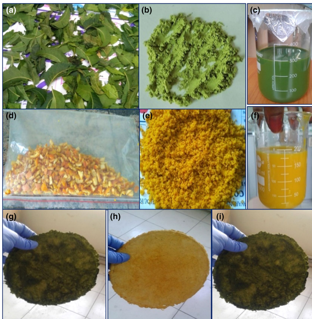
Fig. 2 a Neem leaves, b lyophilized extracted neem, c extracted neem solution, d orange peel, e lyophilized extracted orange peel, f extracted orange peel solution, g neem cotton sheet, h orange cotton sheet, i neem + orange cotton sheet
