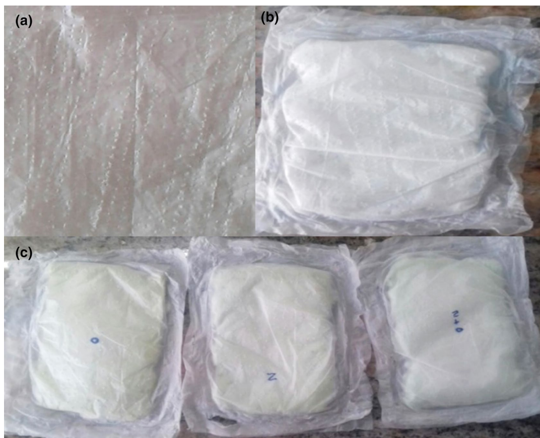
Fig. 3 a Microporous PLA sheet, b microporous PLA covered pure cotton absorbent pad, c microporous PLA covered cotton absorbent pad (orange cotton, neem cotton, orange + neem cotton)
