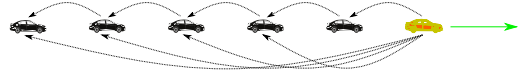
Figure 5: AVFS using information from platoon leader as well as from one vehicle ahead.
