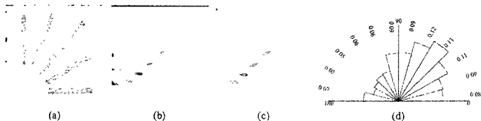
FIG. 4. (a) Test-1 image, (b) Hough/Radon transform, (c) Filtered transform, (d) Rose diagram.
