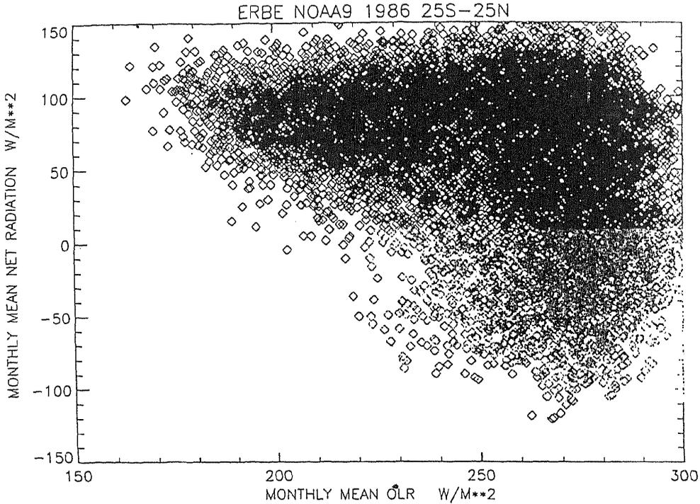
FIG. 10. The variation of monthly mean net radiation with monthly mean outgoing longwave radiation (OLR) in January 1986 from ERBE data (from Srinivasan and Smith, 1996).
