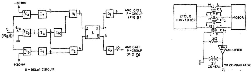
FIG. 10a. Group selection and blanking logic circuit for phase a, b. Current sensing circuit<sup>3R</sup>.
