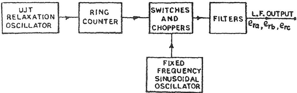
FIG. 8. Block diagram of the variable voltage, variable frequency three phase reference source<sup>38</sup>.
