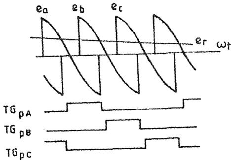
FIG. 4. Deriving firing signals for one group<sup>38</sup>.
