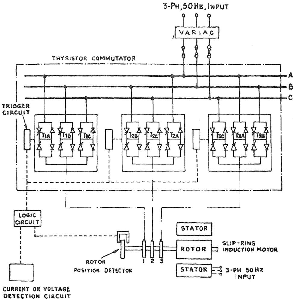
FIG. 14. Cycloconverter-type thyristor commutator motor<sup>20</sup>.
