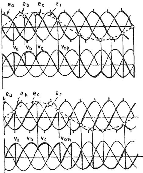
Fig. 6. Derivation of P-group and N-group output voltages.
