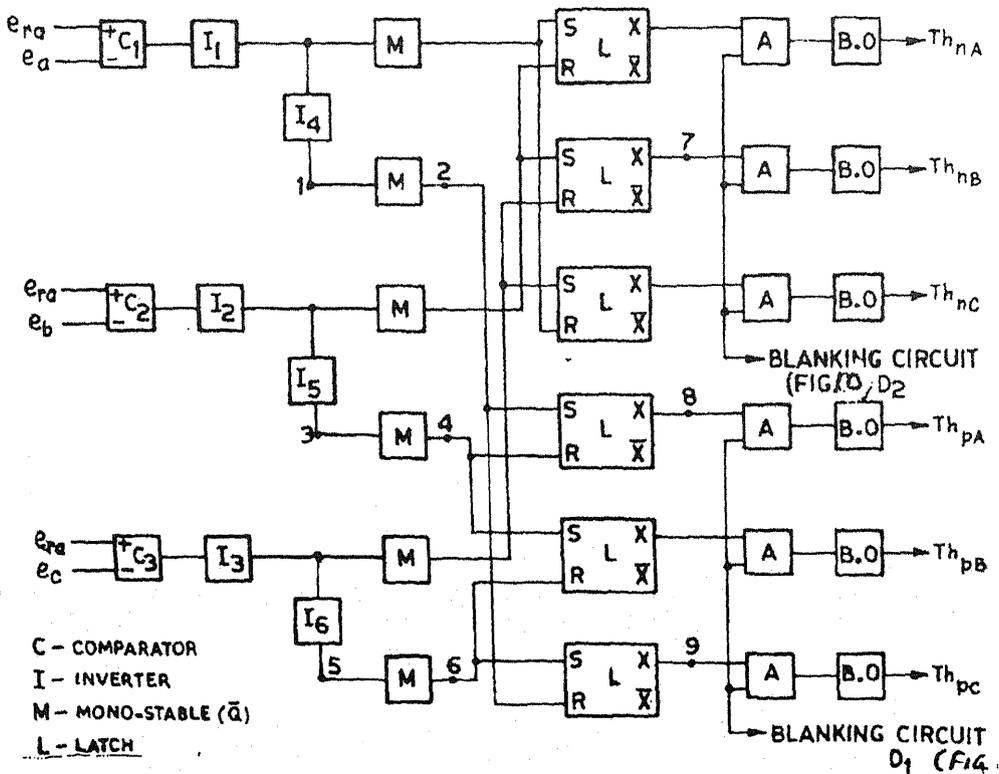
FIG. 9. Block diagram of the main logic and triggering circuit (for phase a of the output only)<sup>38</sup>.
