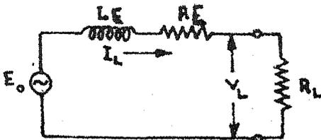
Fig. 19. Cycloconverter equivalent circuit<sup>79</sup>,  $R_E = (p/2\pi)\omega_s L$ ;  $L_E = L$ ;  $E_o = KE_{db} \sin \omega_s t$ .
