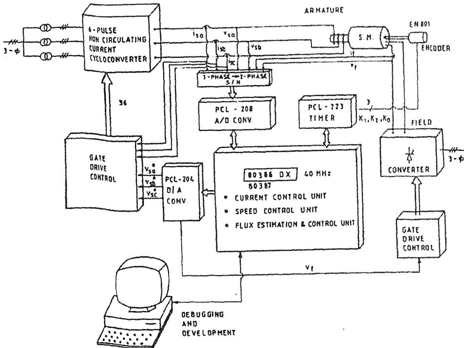
Fig. 13. Hybrid implementation of a cycloconverter-fed synchronous motor with a 386 PCAT<sup>71</sup>.
