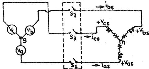
Fig. 20. Representation of induction motor with switchings in the stator<sup>83</sup>.
