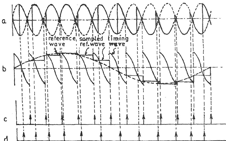
FIG. 12. Cycloconverter operation with regular sampling [26].
