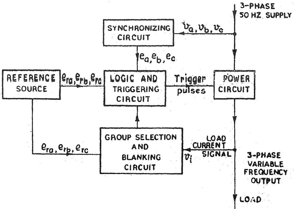
Fig. 7. Block diagram for a circulating current-free cycloconverter control circuit.<sup>38</sup>
