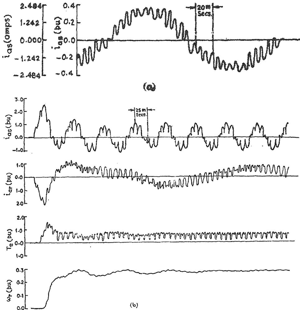
FIG. 21a. Digitally computed steady-state current waveform for 5 Hz. b. Dynamic performance of induction motor with 3-pulse cycloconverter. Digital simulation results.  $f_s = 16$  Hz,  $k_r = 0.806$ ,  $V_r = 0.5$  pu,  $T_L = 0.5$  pu (Non-circulating current mode)<sup>83</sup>.
