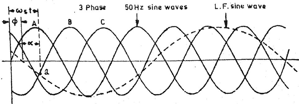
FIG. 5. Derivation of cosine modulating voltages<sup>40</sup>.
