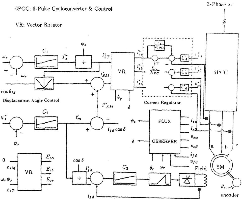
FIG. 16. Block diagram of the stator flux oriented vector control scheme with flux observer for a cycloconverter-fed synchronous motor<sup>71</sup>.
