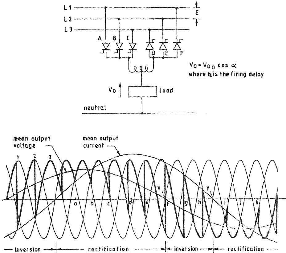
Fig. 1. Output voltage waveform for one phase of a three phase cycloconverter operating at 15 Hz from 50 Hz supply, 0.6 p. f. lagging load<sup>30</sup>.
