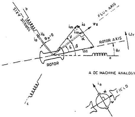
Fig. 17. Space phasor diagram of a vector controlled synchronous motor<sup>34</sup>.
