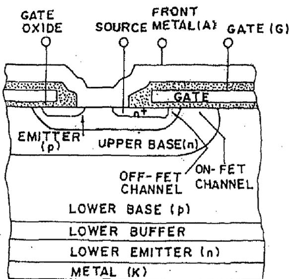
FIG. 2. Cross-sectional view of a p-MCT cell.
