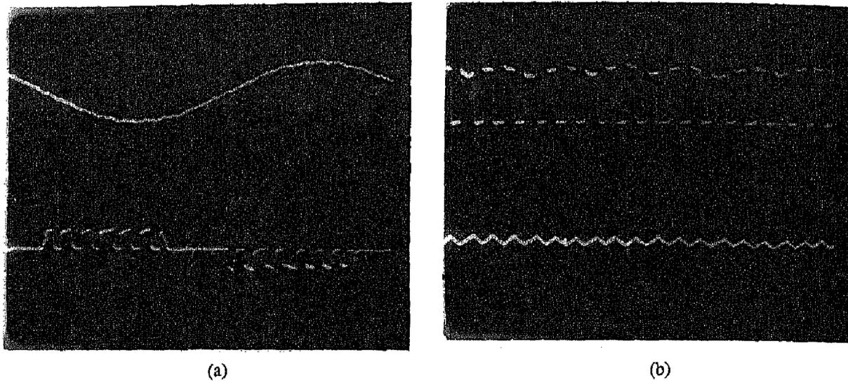
FIG. 9. Input and output waveform of the MCT based AC/DC converter circuit. (a) Upper :  $V_{LL}$ (100V/div); Lower : Input current(5A/div); Time : 2 msec/div; (b) Upper : Output voltage (50V/div); Lower : Output current (5A/div); Time : 2 msec/div.
