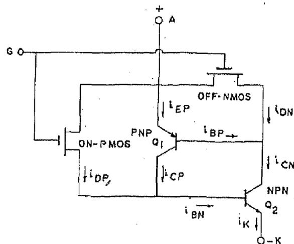
FIG. 3. Equivalent circuit of a p-MCT cell.
