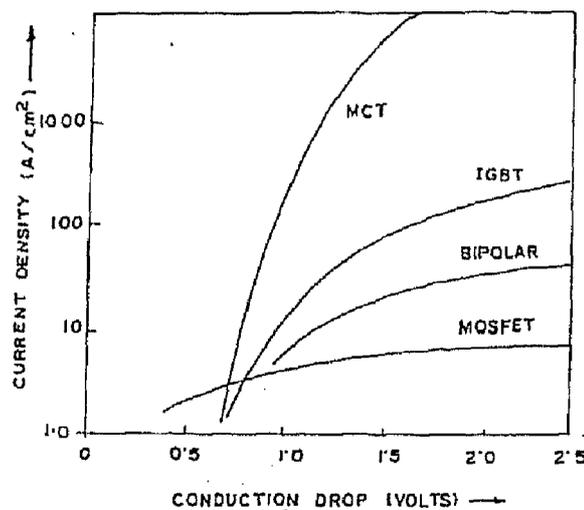
FIG. 1. Comparison of on-state voltage drop of different power devices.
