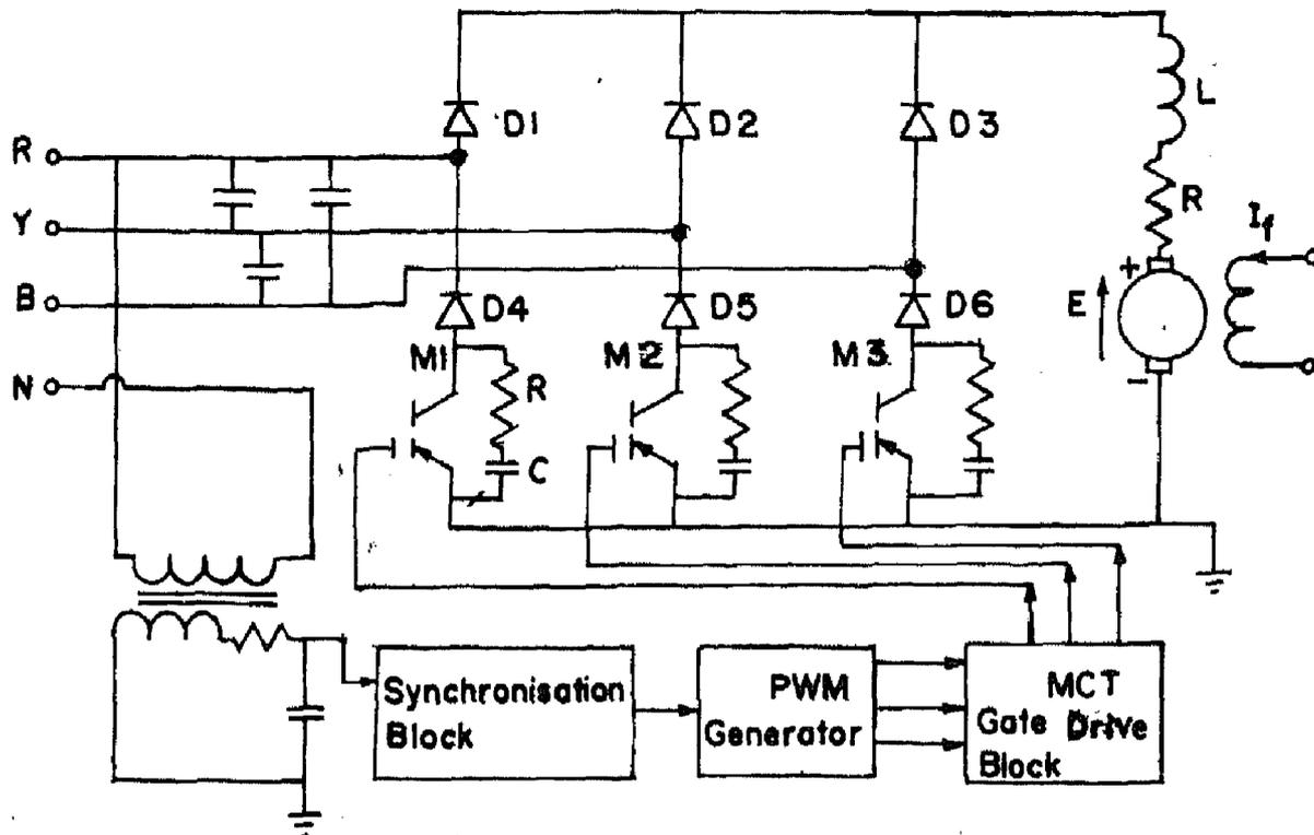
FIG. 8. Schematic diagram of the PWM AC/DC converter circuit using MCT.
